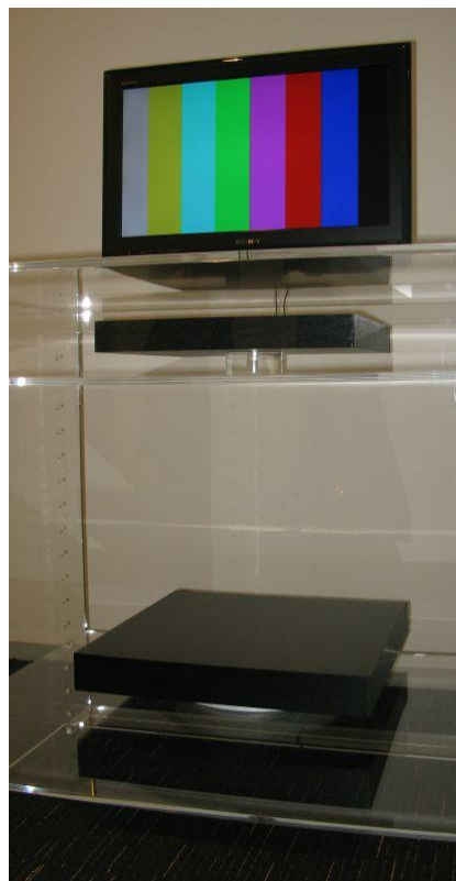
Fig.1.8 Demonstration by SONY (Air gap: 50[cm], Efficiency:80[%])
