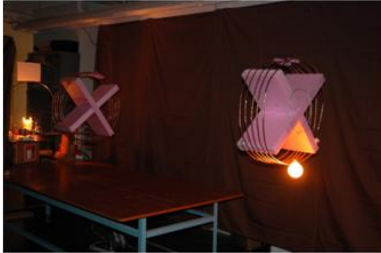
Fig.1.4 Demonstration by MIT group (Air gap:2[m], Power:60[W])
