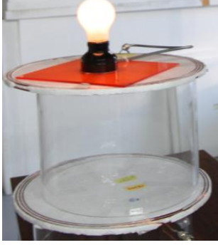
Fig 2.2. Wireless power transfer via MRC using the prototype resonator pair used in this study.
