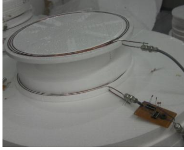
(i) Resonator pair with IM circuit connected to transmitting resonator (a) Photo of resonator pair and IM circuit used in manual matching experiment.
