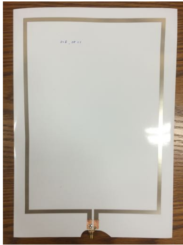
(a) Overprinted coupling coil
