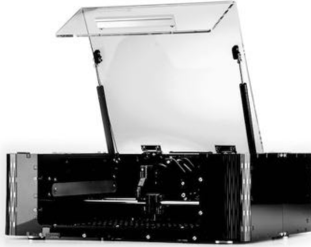
Fig. 3.1: Argentum - a printer used to print conductive material for fabrication of circuit boards [8]
