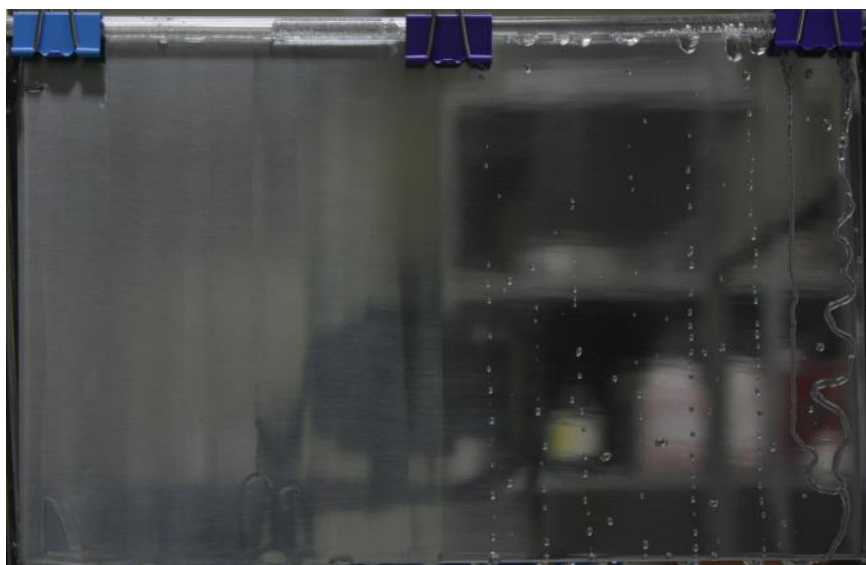
(a) Formation of water film w/ nano particle coating (left) and w/o the coating (right)
