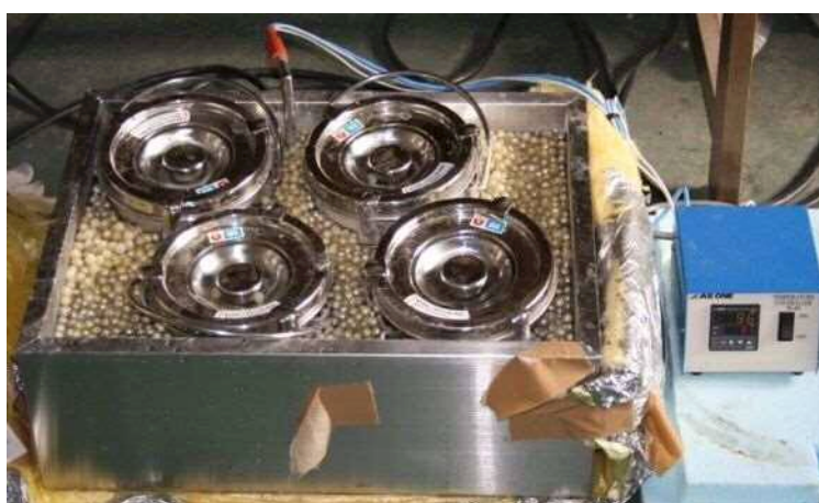
Fig. 4.9 External view of the canisters kept thermally-steady at 95 °C.
