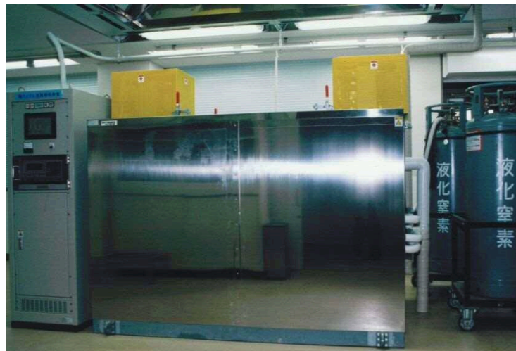
Fig. 3.2 External view of thermal cycle apparatus.
