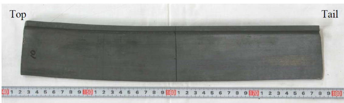
Fig. 5-5 Example of rolled pure lead specimen ( r_w=15.6\% , r_f=17.8\% )
