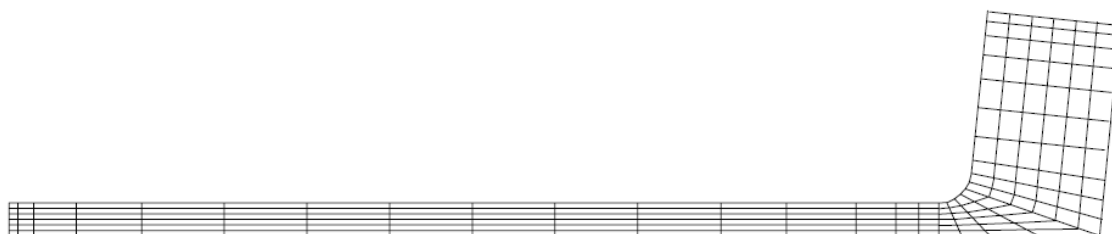
Fig. 3-10 Elements in the section (thick section)
