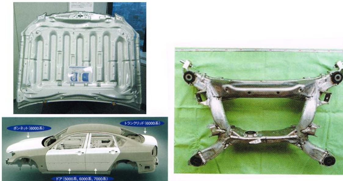
Fig.1.21 Front hood, door panel and sub-frame [1-36][1-37] .
