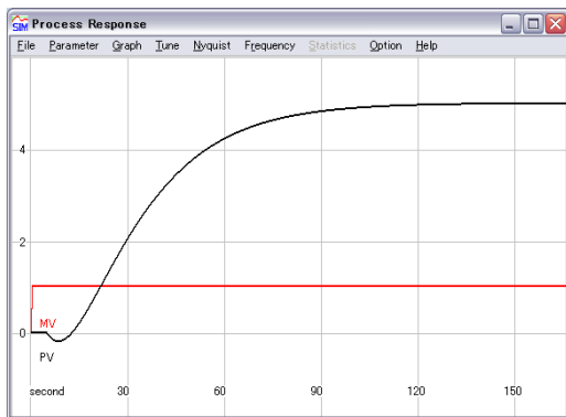
(a) Step responses of a integral process with dead time ,where PV in Black line and MV in Red Line
