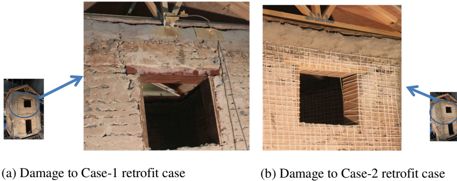
Figure 6-9: Comparison of Cracks at Run 21 (25 HZ, 0.2g)
