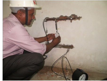
(b) Setting of dial gauge for deformation measurement
