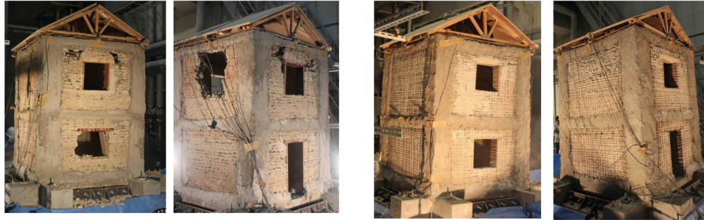
(a) Damage to case-1 retrofit case
