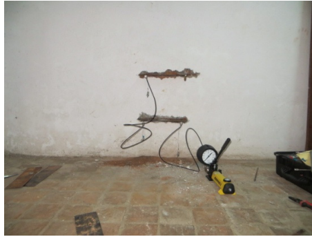
(a) Flat jacks inserted in the cut slits
