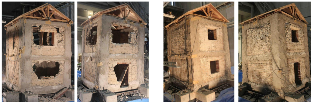
(a) Damage to case-1 retrofit case
