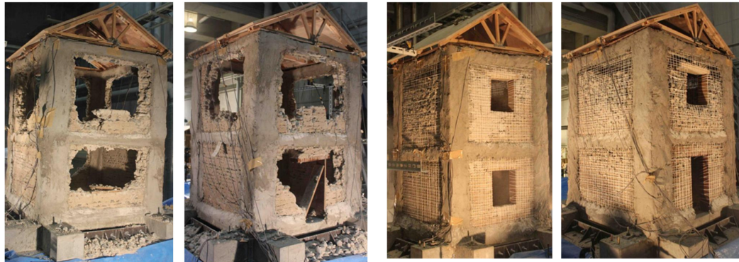
(b) Damage to Case-2 retrofit case
