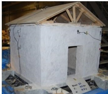
(a) Photo of experimental model house under test (Photo from Sakurai, K., 2011)
