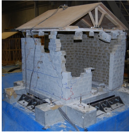
Figure 4-8: Door side photo after run 45 (5HZ-0.6g) of experiment (Sathiparan, N. 2008)
