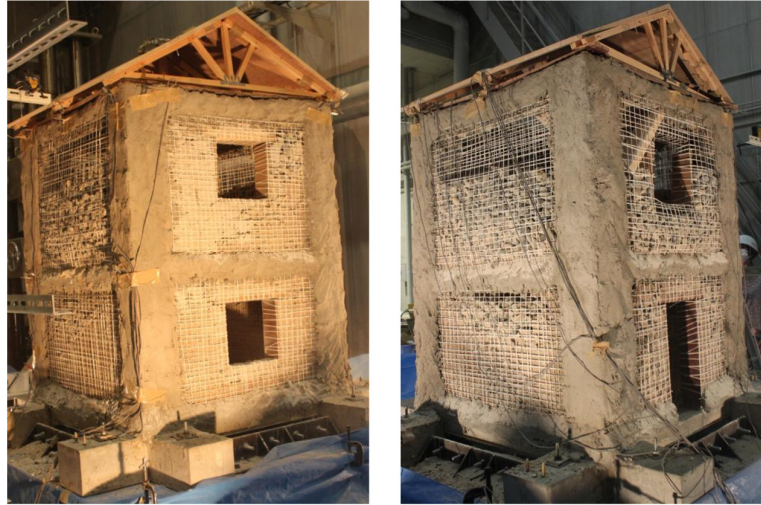
Figure 6-15: Level of Damage at Run 42 for Case-2 Retrofit
