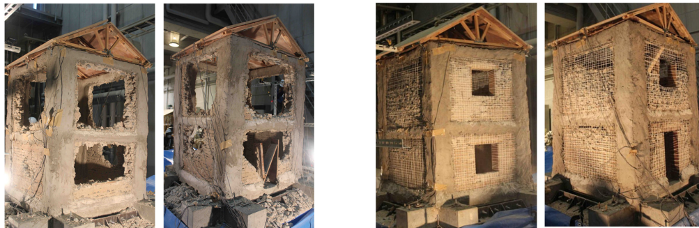
(a) Damage to Case-1 retrofit case
