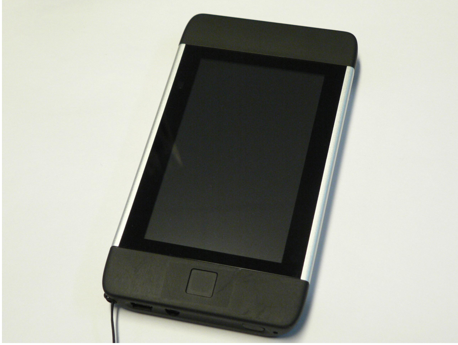
Figure 4.12: The mobile terminal for on-line calculation of its relative position to the vehicle.
