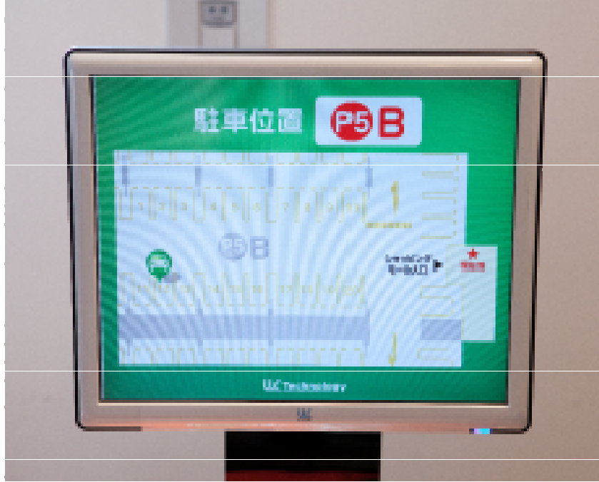
Figure 6.5: Digital signage shows the position of the vehicle when the user entered the ID of the parking pass to the signage unit.
