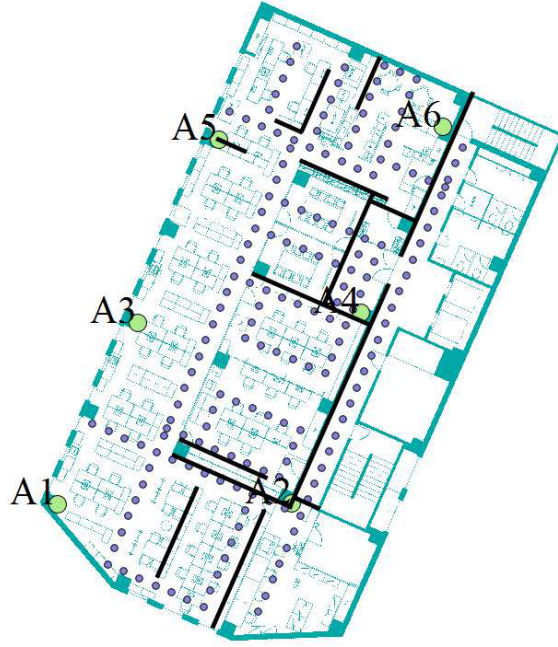
Figure 5.6: The layout of the office. Positions of tags are marked with alphabets. Black lines represent metallic objects in the office.
