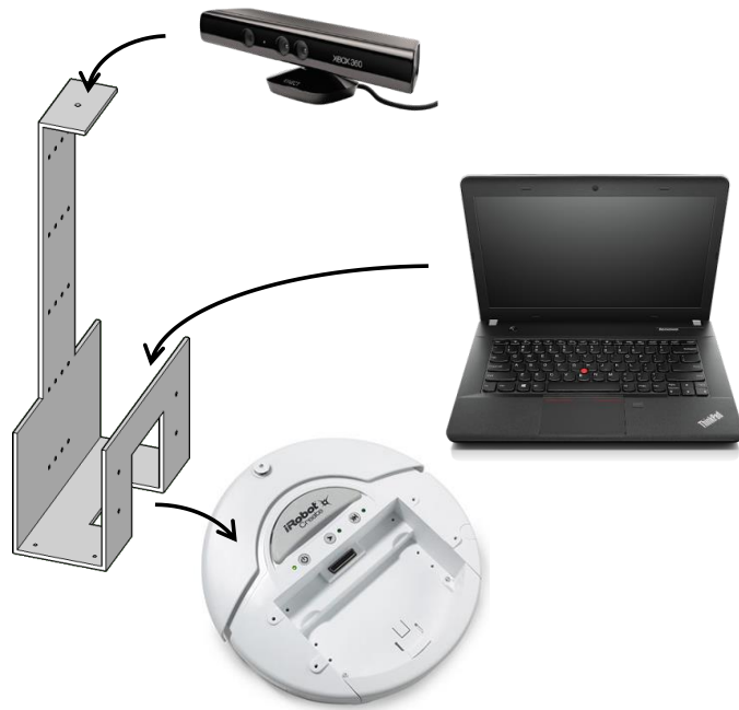
Figure 6.1: Hardware components: iRobot Create mobile base, laptop, Microsoft Kinect Xbox 360 and acrylic body frame.
