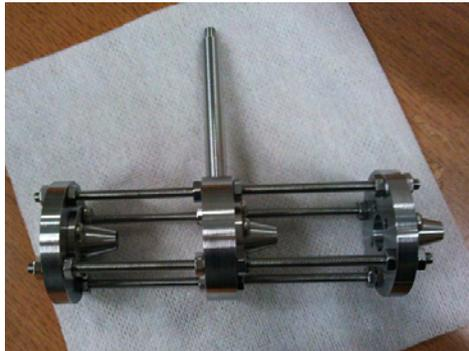
Figure 3.20: A photograph of the baffle at the exit of the velocity map imaging chamber.
