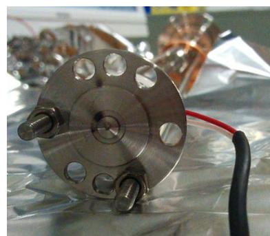
Figure 3.12: A photograph of the nozzle of the pulsed valve for sample gases.
