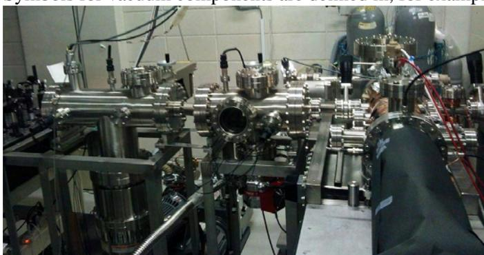
Figure 3.11: A photograph of the chambers used in the experiment. Left: harmonic generation chamber. Middle: refocusing chamber. Right: detection gas source chamber (far side) and velocity map imaging chamber (near side). The grating spectrometer is not shown.
