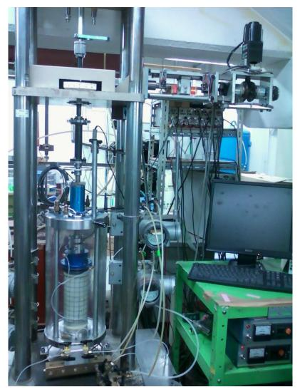
Figure 4.6. Hollow cylinder torsional shear device
