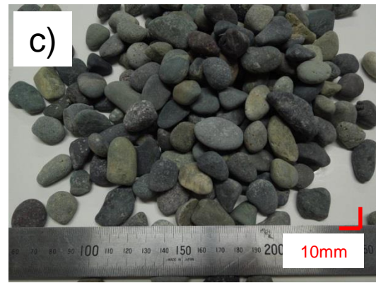
Gravel No.5 ( D_{50}=14.2\text{mm} )
