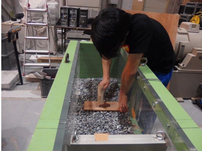
Fig. 3.20 Manual hand-held plate compaction method for gravel
