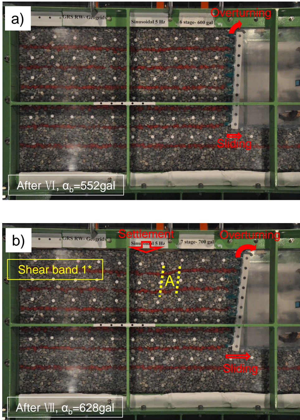
Fig. 5.9 Deformation modes of geogrid M -RS RW-G: a) after shaking stage VI ( \alpha_b = 552 gal); b) after shaking stage VII ( \alpha_b = 628 gal);
