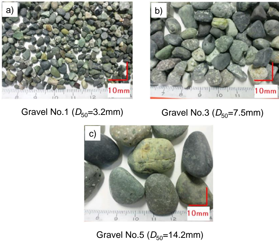
Fig. 3.5 Backfill materials used in this study a) Gravel No.1; b) Gravel No.3; c) Gravel No.5.
