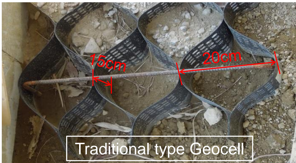
Fig. 2.2 Traditional diamond-shaped geocell
