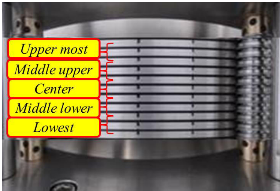
Fig. 5.31: Sections of the 11 non-coated stacked rings used for image analysis
