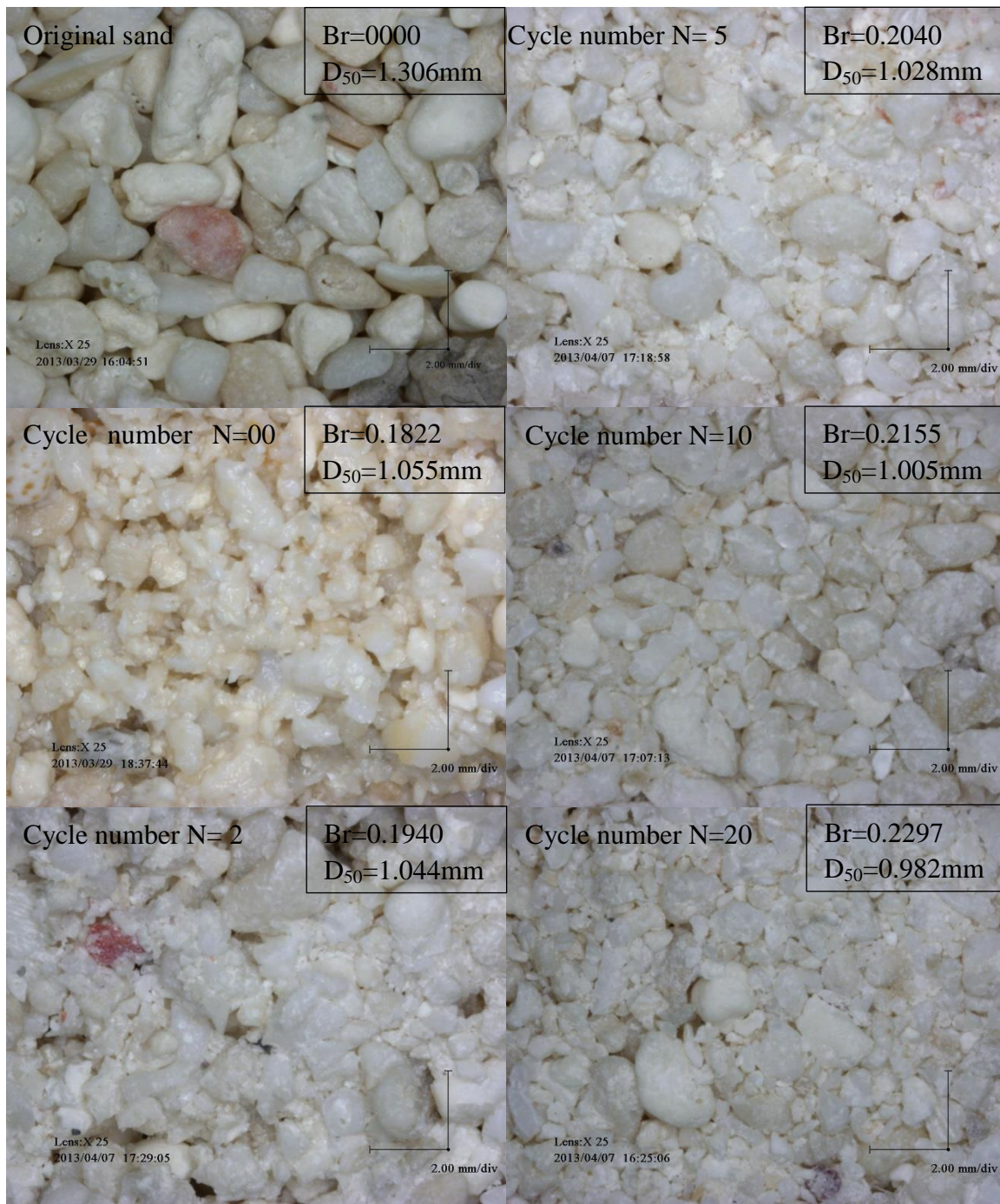
Figure 6.5 Microscopic view on particle breakage from CD tests subjected to cyclic loading ( \sigma_c=3\text{MPa} K_0=1.0 e_0=0.798 )
