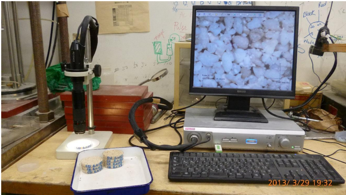
Figure 6.1 Microscope equipment with 186-time lens in maximum
