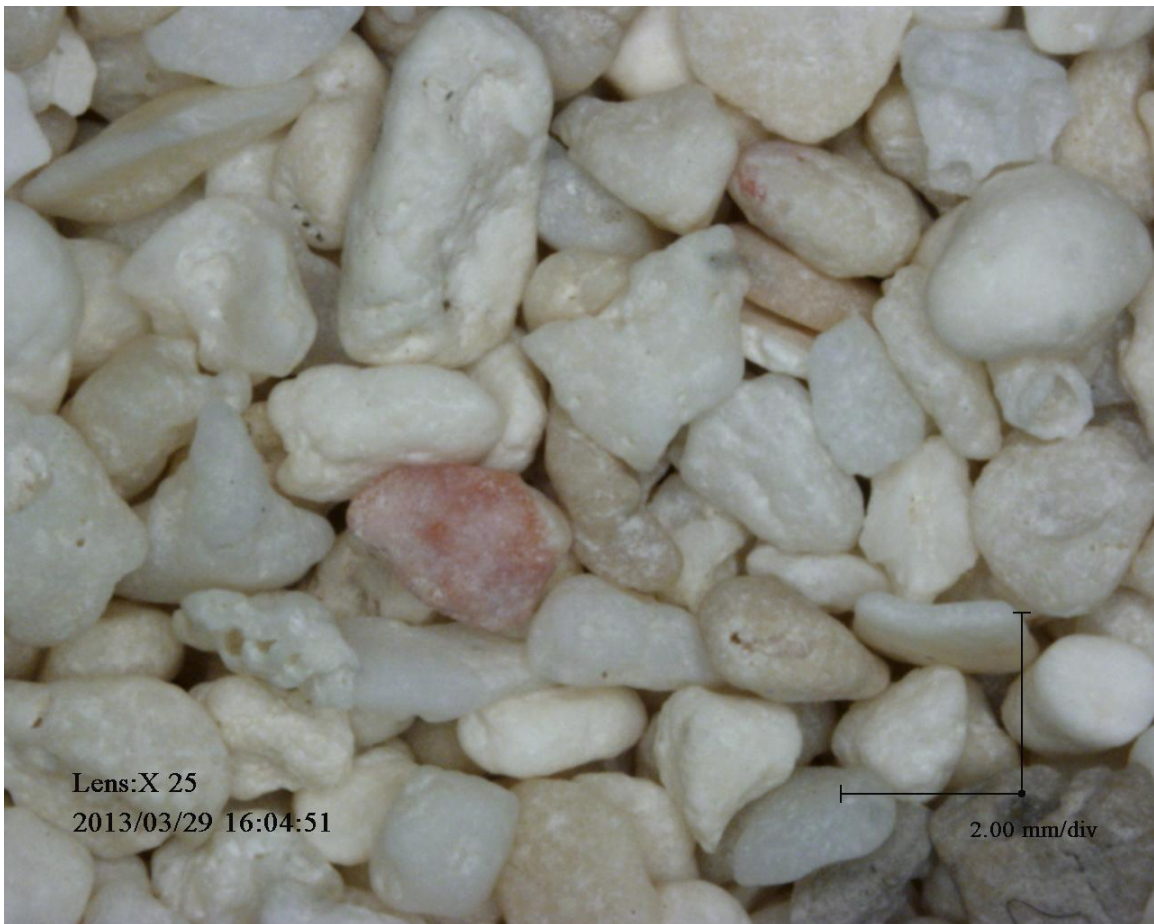
Figure 6.2 Microscopic view on original Coral sand No.3
