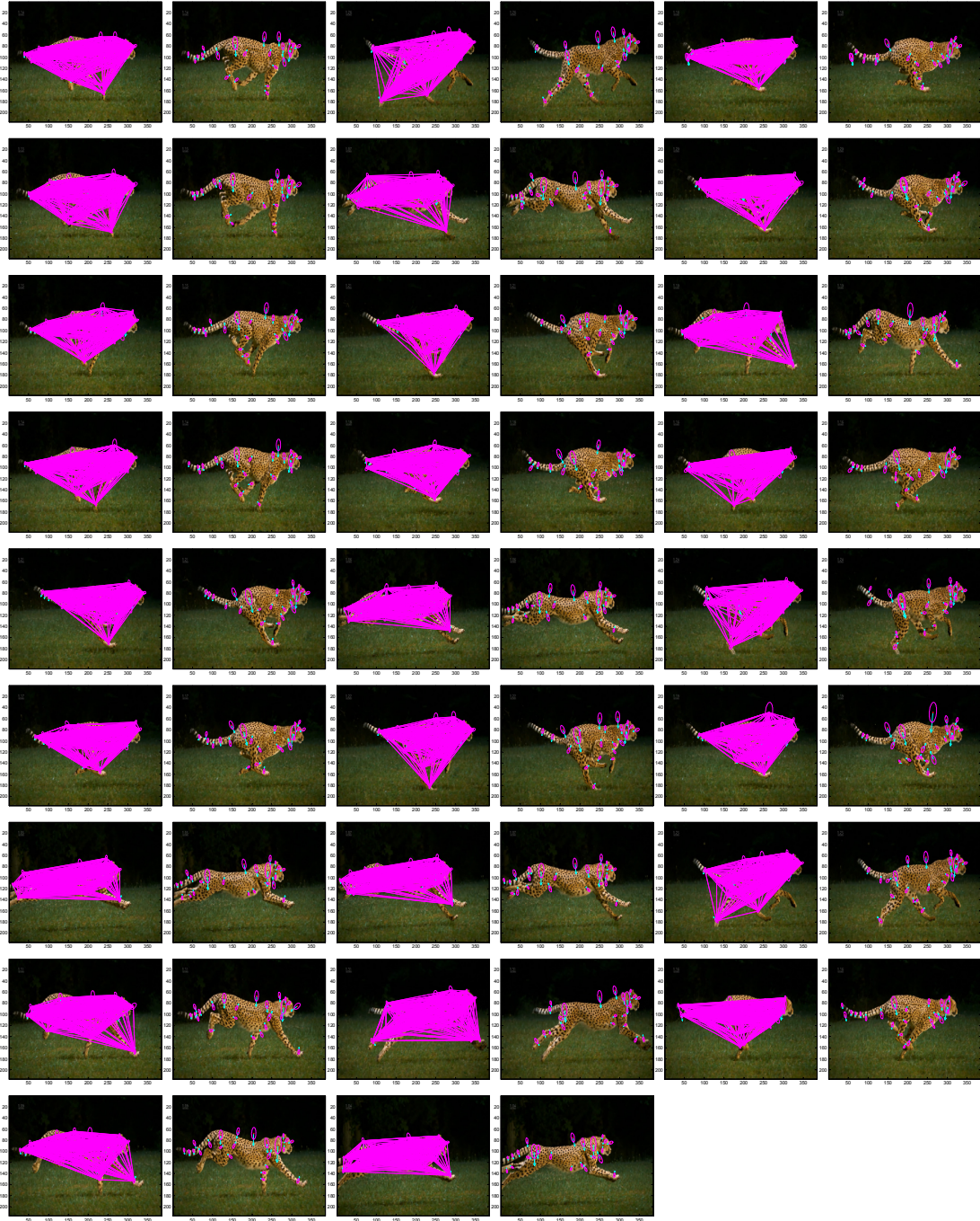
Figure 6.3: Detection of the cheetah in video frames based on the trained deformable model.
