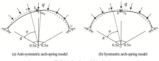
Fig.E-1 Arch-spring models in-plane
