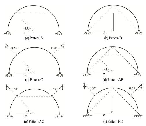
Fig.E-3 Stiffening patterns of single arch in-plane
