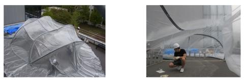
Fig.7-18 Buckling of skeletons of rectangle shelter in April (≈-30Pa)
