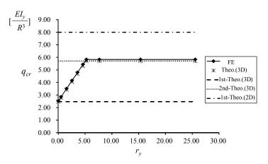
Fig.5-13 Relationship of  $r_y$  and  $q_{cr}$  with fixed ended boundaries in-plane
