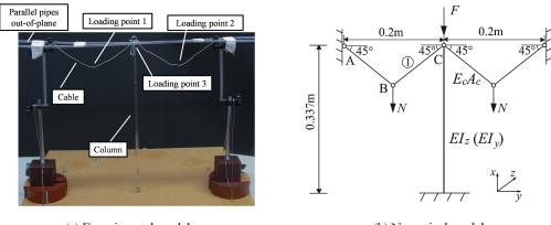
(a) Experimental model (b) Numerical model Fig.7-37 Experimental model and numerical model
