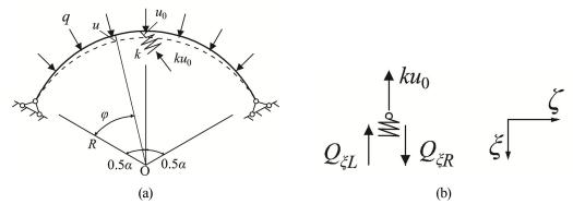
Fig.5-11 Arch-spring model out-of-plane
