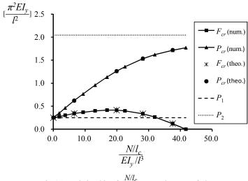
Fig.6-15 Relationship of  $\frac{N/l_c}{EI_V/l^3}$ ,  $F_{cr}$  and  $P_{cr}$  out-of-plane
