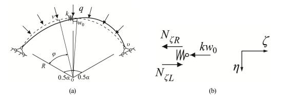
Fig.5-1 Anti-symmetric arch-spring model
