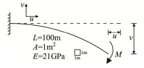
Fig.3-6 Cantilever beam under bending moment<sup>[159]</sup>
