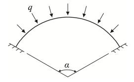
Fig.4-1 Circular arch under uniform compression
