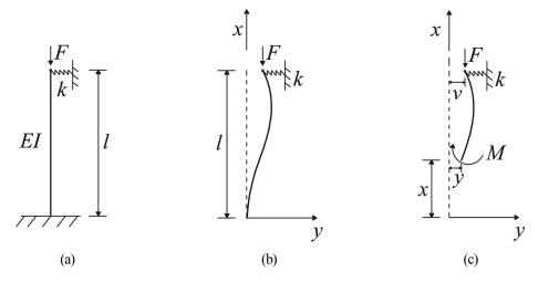
Fig.C-3 Column stiffened by one spring at top
