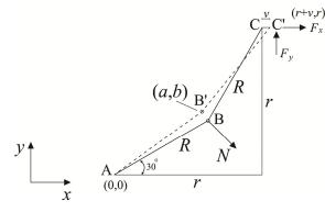
Fig.D-1 Mechanistic movement of the membrane
