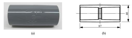
Fig.7-4 Joint of PVC pipes
