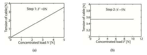
Fig.6-11 Relationship of tension of cable with N and F
