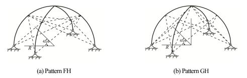
Fig.5-23 Two hybrid stiffening patterns of cross arch
