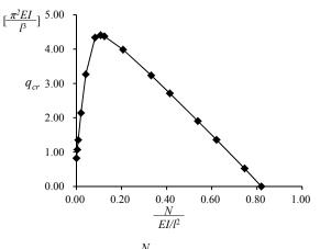
Fig.6-19 Relationship of  $\frac{N}{EI/l^2}$  and critical distributed load  $q_{cr}$
