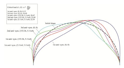
Fig.5-10 Variation of anti-symmetric modes with fixed ended boundaries
