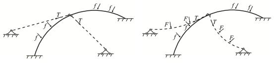
(a) Component stiffening method (b) External force stiffening method
