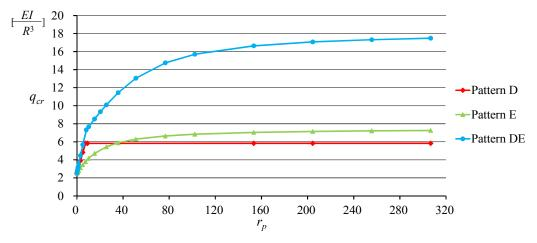
Fig.5-21 Relationship of  $r_p$  and first order critical loads  $q_{cr}$
