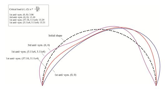
Fig.5-7 Variation of anti-symmetric modes with hinged ended boundaries
