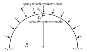
Fig.5-4 Numerical model of the arch in 2D plane
