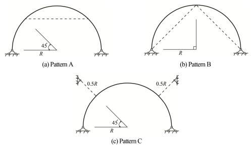
Fig.5-14 Three basic stiffening patterns in-plane
