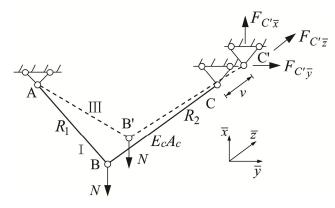
Fig.6-5 Mechanistic movements of curved cables out-of-plane
