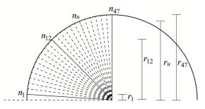
Fig.D-2 Heights of nodes in the circular arch
