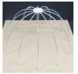
Fig.7-1 Miniature model of hemispheric shelter
