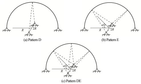
Fig.E-4 Stiffening patterns of single arch out-of-plane
