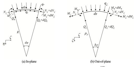
Fig.B-5 Isolated infinitesimal body of the arch (in Chapter 4)  $^{[108]}$
