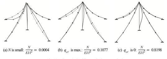
Fig.6-20 First order buckling modes by FE method
