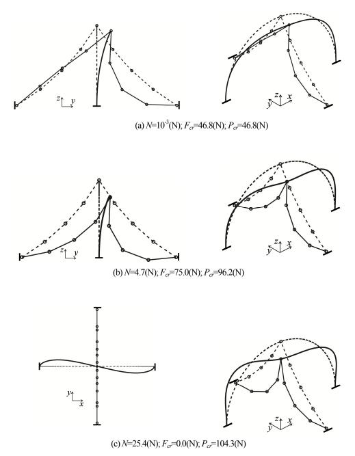
Fig.6-26 First order buckling modes of the arch with curved cables
