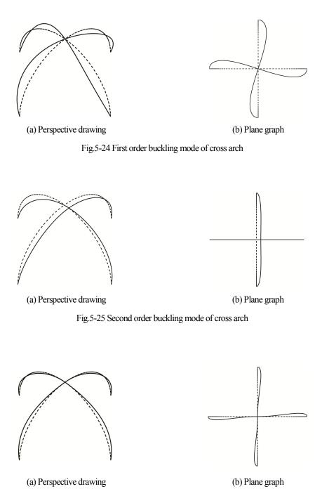
Fig.5-26 Third order buckling mode of cross arch
