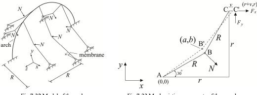
Fig.7-32 Model of the arch
