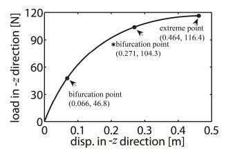
Fig.6-23 The relationship of displacement and load in -z direction
