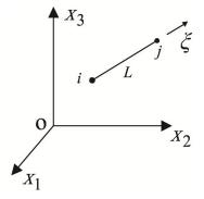
Fig.3-3 Truss element in 3D space [151]
