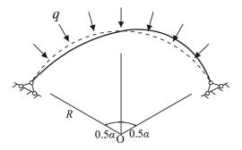
Fig.4-5 Buckling of the arch in-plane
