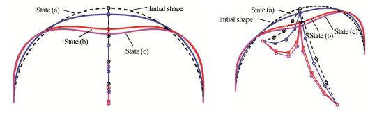
Fig.6-25 Equilibrium shapes of the arch before buckling
