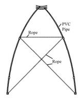
Fig.7-5 Setting of stiffening rope
