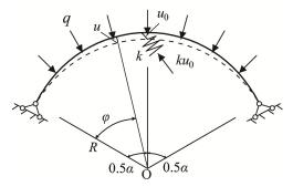
Fig.E-2 Arch-spring model out-of-plane
