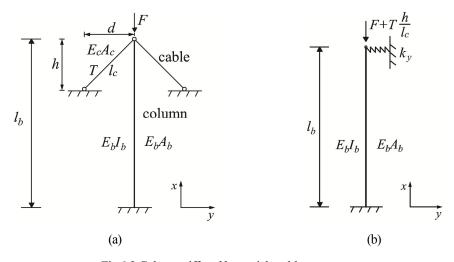
Fig.6-2 Column stiffened by straight cables
