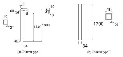
Fig.7-24 Two types of columns
