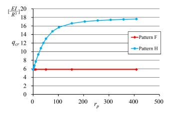
Fig.5-31 Relationship of  $r_p$  and the first order critical load  $q_{cr}$  (fixed ended boundaries)
