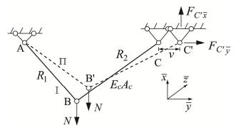
Fig.6-4 Mechanistic movements of cables in-plane
