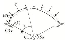
Fig.4-10 Buckling of the arch out-of-plane
