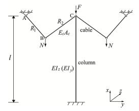
Fig.6-3 Column stiffened by curved cables
