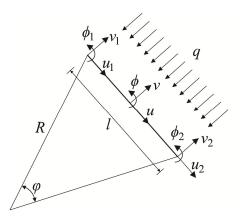
Fig.3-4 A straight beam element for the circular arch/ring [74]
