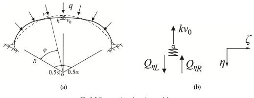
Fig.5-2 Symmetric arch-spring model
