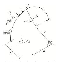
Fig.6-21 Arch featuring with curved cables
