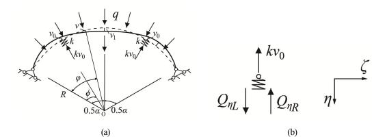
Fig.B-3 Circular arch with hinged ended boundary conditions
