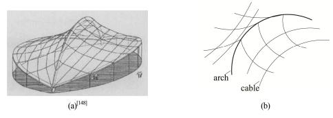
Fig.1-4 Arch structures supported by cable-nets
