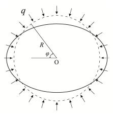
Fig.5-33 Buckling problem of ring in-plane
