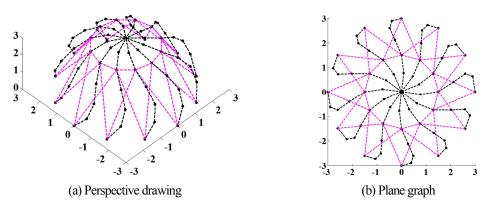
Fig.7-12 First order buckling mode with ropes (First order critical load=-44.0Pa)
