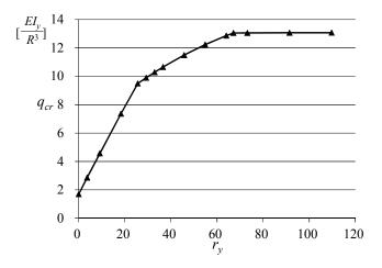
Fig.5-35 Relationship of parameter  $r_y$  and the first order critical load  $q_{cr}$
