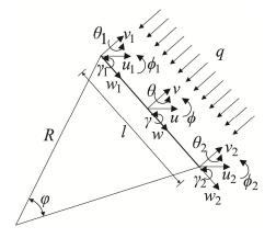
Fig.3-5 A straight beam element for a circular arch/ring
