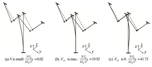
Fig.6-16 First order buckling modes out-of-plane by n FE method
