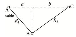
Fig.6-6 Initial geometric shape of curved cables
