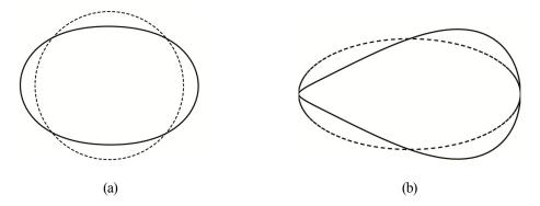
Fig. 5-34 First order buckling modes in-plane and out-of-plane
