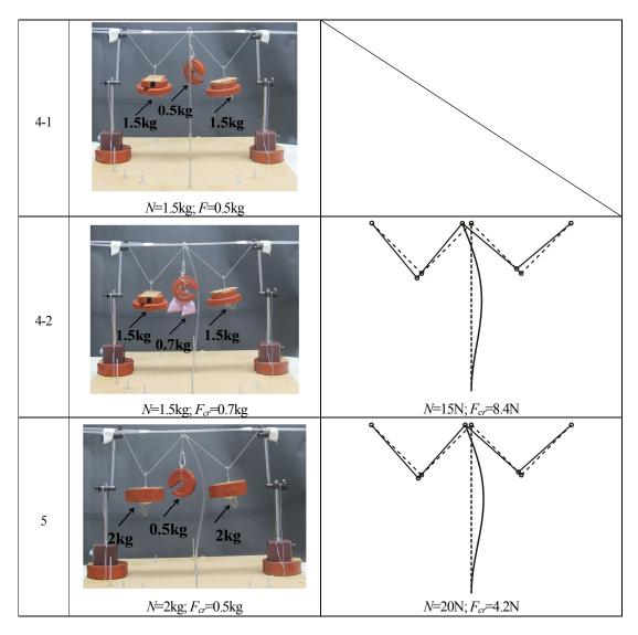
Table.7-4 shows the comparison of results of the critical loads and buckling modes in experiment and FE analysis. From Table.7-4, the buckling modes in experiment and numerical examples can be observed to be very similar to each other.
