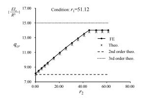
Fig.5-5 Comparison of the results with hinged ended boundaries
