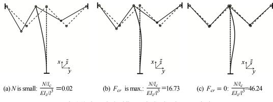
Fig.6-13 First order buckling modes in-plane by FE method
