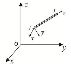
Fig.3-1 Global and local Cartesian coordinate system of 3D-beam element
