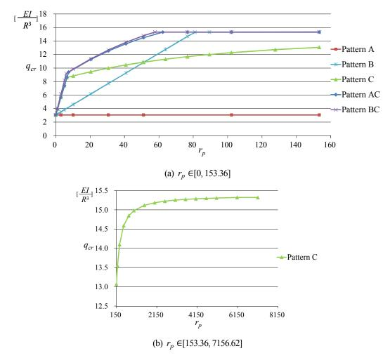
Fig.5-16 Relationship of  $r_p$  and first order critical load  $q_{cr}$  (hinged ended)
