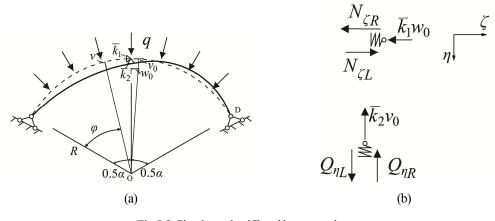
Fig.5-3 Circular arch stiffened by two springs
