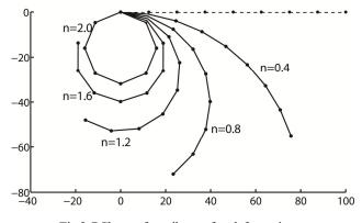
Fig.3-7 Shape of cantilever after deformation
