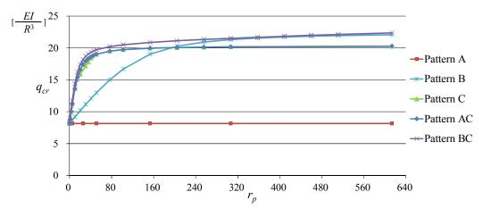
Fig.5-17 Relationship of  $r_p$  and first order critical load  $q_{cr}$  (fixed ended)
