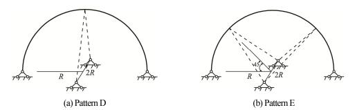
Fig.5-18 Two basic stiffening patterns out-of-plane
