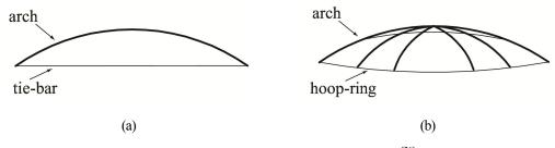
Fig.1-2 Arches with components in the boundary [26]
