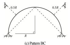
Fig.5-15 Three hybrid stiffening patterns in-plane
