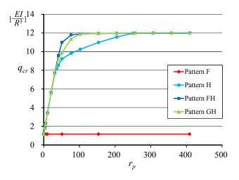
Fig.5-27 Relationship of  $r_p$  and first order critical load  $q_{cr}$  (hinged ended boundaries)
