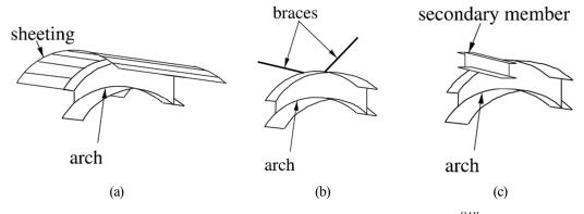
Fig.1-1 Constraint components at local places of the arch structures [144]
