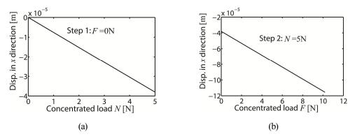
Fig.6-10 Relationship of displacement with N and F
