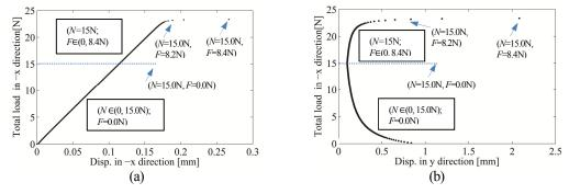
Fig.7-38 Relationship of displacement and total load
