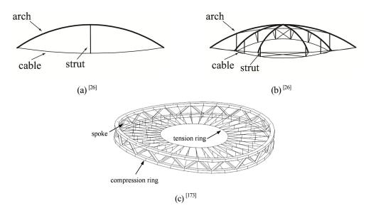
Fig.1-3 Arch with components at boundary
