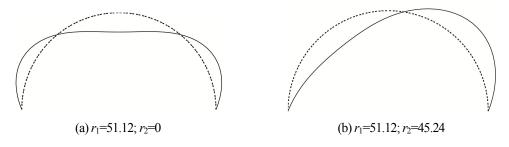
Fig.5-6 First order buckling modes ( $r_1$ =51.12)
