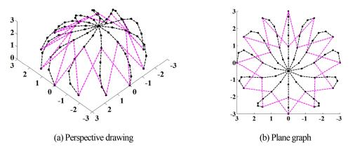
Fig.7-13 First order buckling mode with ropes (First order critical load=-25.2Pa)
