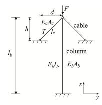
Fig.C-1 Column stiffened by straight cables [174]
