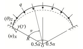
Fig.4-11 Buckling of the arch out-of-plane
