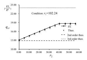
Fig.5-8 Comparison of the results with fixed ended boundaries
