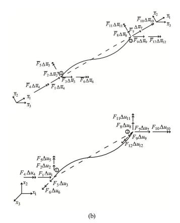
Fig.3-2 Displacements and internal forces of beam element [86], [101]
