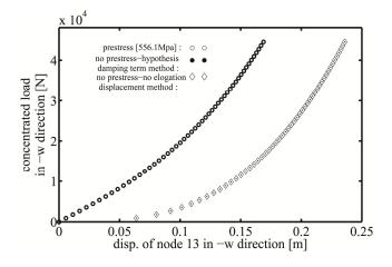
Fig.A-2 Relationship of displacement and concentrated load
