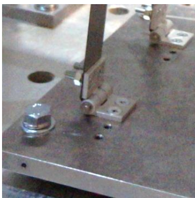
a) Original pinned connection
