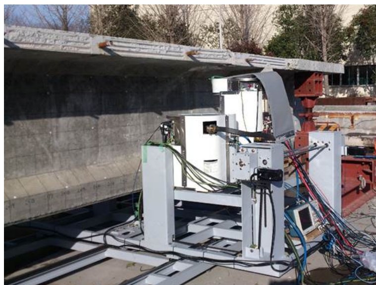
FIGURE 2.11: 950keV Linac on the stage frame
