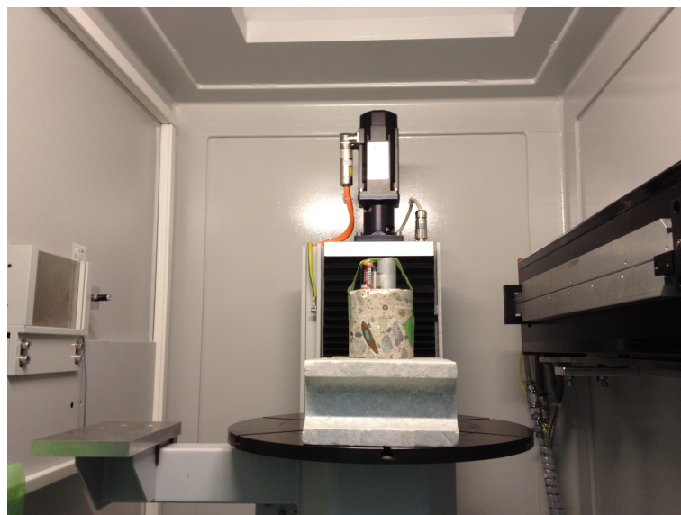
FIGURE 4.3: Small concrete sample in compact CT device
