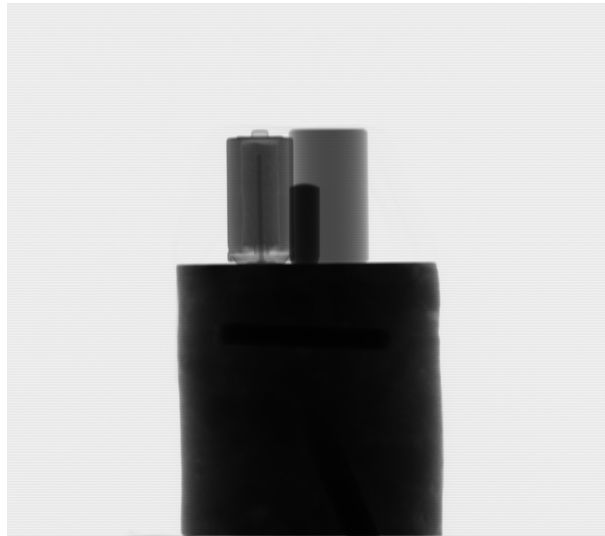
FIGURE 4.4: Transmission image of small concrete sample by compact CT device
