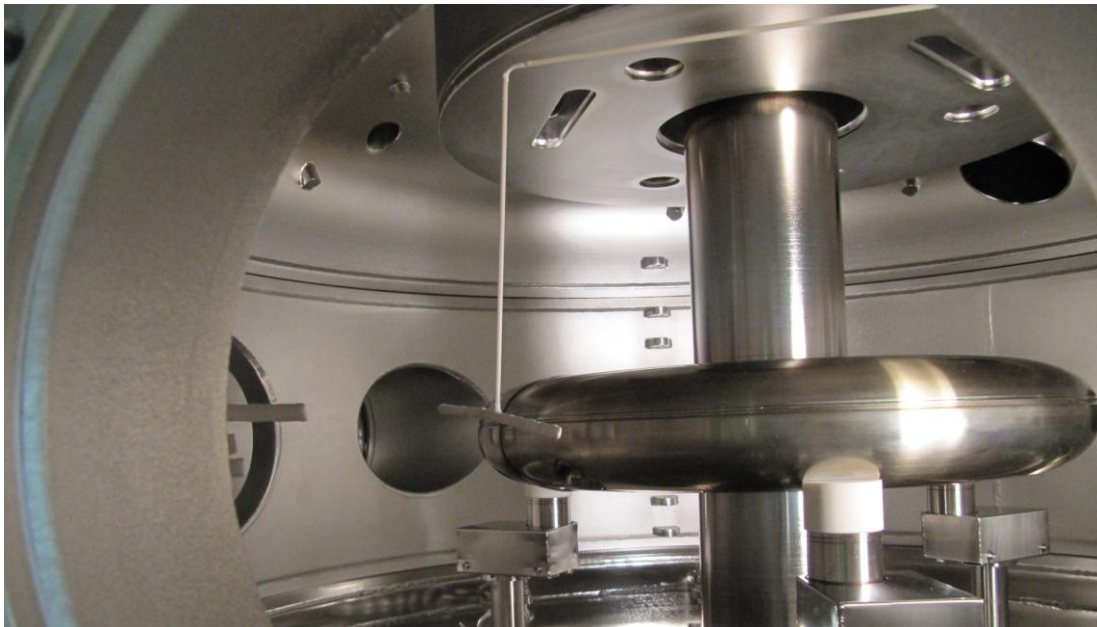
Figure 5.12: A photograph of installed SX-B antenna
