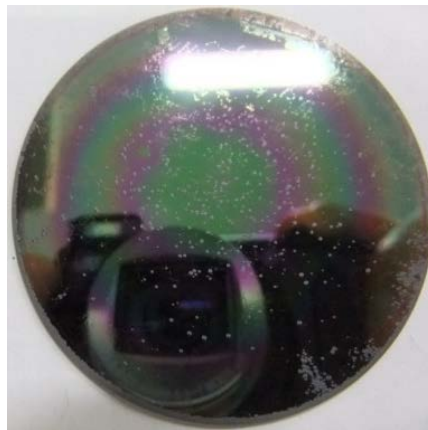
Fig. 2.8 GaN surface with Si melt-back spots, grown in a clean reactor, with all new parts.
