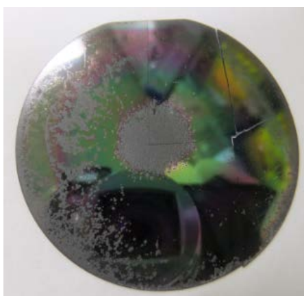
Fig. 2.9 Surface of GaN grown on Si without cleaning.
