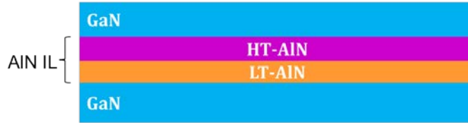
Fig. 6.4 Structure of HT/LT-AlN two-step interlayer.
