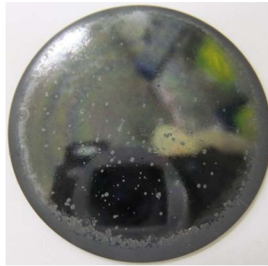
Fig. 2.13 Surface of GaN on \text{NH}_3 pre-flowed Si surface.
