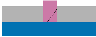
Figure 6: Extinction of threading defect in selective area growth.
