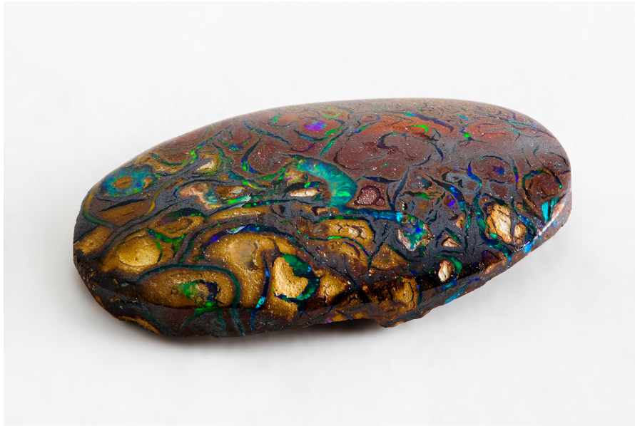
Figure 28: Opal gemstones owe their brilliant colors to natural photonic crystal structures. (Photo by J.J. Harrison [9].)
