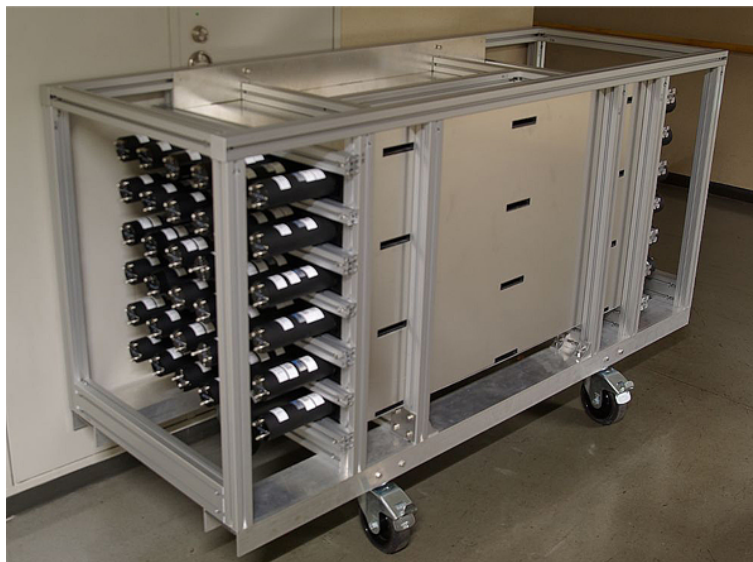
Figure 3.4: PANDA36: The prototype of the PANDA detector, which consists of 36 modules
