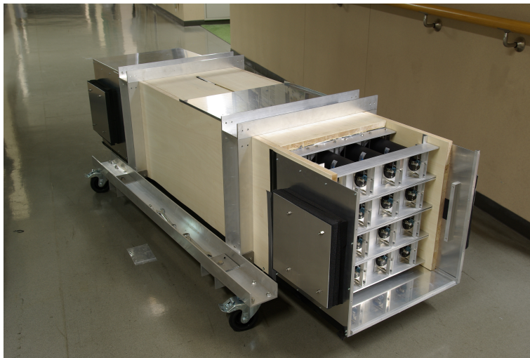
Figure 3.3: Lesser PANDA: A prototype of the PANDA detector, which consists of 16 modules
