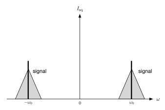
Fig. 4.3 The signal power spectrum of AC-biased TES
