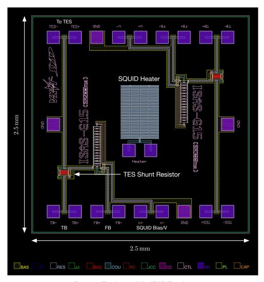
Fig. 3.4 The design of the ISAS-G15 chip
