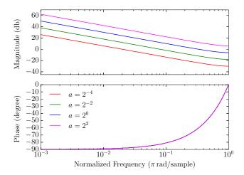
Fig. 4.10 Frequency responses of discrete-time integrator for various gains
