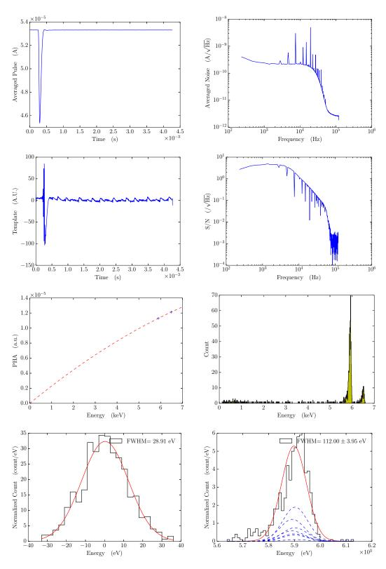
Fig. 5.17 The 4-channel simultaneous pulse collection result in channel 1 at  $170\,\mathrm{mK}$ : the averaged pulse (top left), the averaged noise (top right), the template (2nd top left), the signal-to-noise ratio (2nd top right), the energy calibration curve (2nd bottom left), the energy spectrum (2nd bottom right), the baseline energy resolution (bottom left), and the energy resolution at  $\mathrm{MnK}\alpha$  (5.9 keV).
