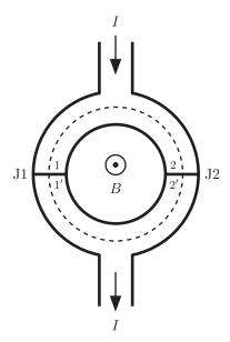
Fig. 2.14 The integral path on the superconducting ring of dc SQUID
