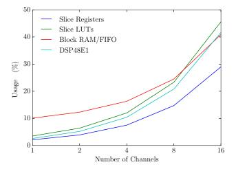
Fig. 4.20 Resource utilization for various number of channels
