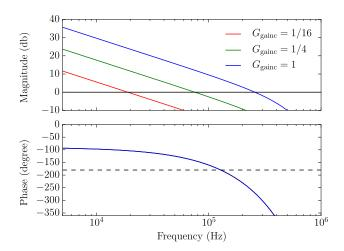
Fig. 4.15 Overall gain in the digital electronics for various gain parameters ( $G_{\text{div}} = 1$ )
