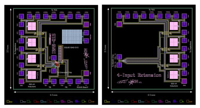
Fig. 3.5 The designs of the 4-input ISAS-G15 chip with inductors (left) and the 4-input extension chip with inductors (right)
