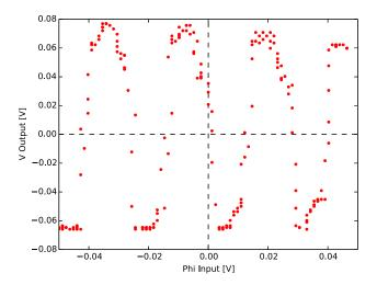
Fig. 5.7 The  $\Phi$ -V curve ( $I_{\rm SB}=17\,\mu{\rm A}$ ) at 200 mK and the operating point during the measurements
