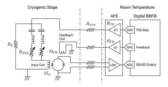
Fig. 6.1 A typical experimental setup for a FDM TES readout
