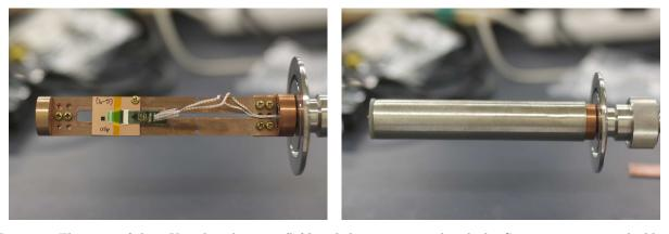
Fig. 3.15 The stage of the 4 K probe: the stage (left) and the stage covered with the Cryoperm magnetic shielding
