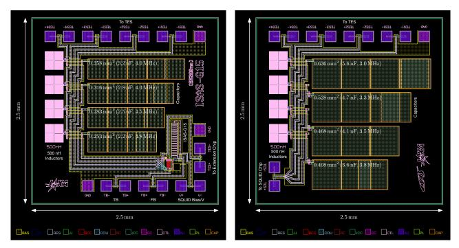
Fig. 3.7 The designs of the 4-input ISAS-G15 chip with built-in LC filters and the 4-input extension chip
