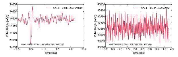
Fig. 6.6 The observed crosstalks: the possible thermal crosstalk in the non-multiplexing pulse collection (left) and the electrical crosstalk in the 4-channel simultaneous pulse collection (right)
