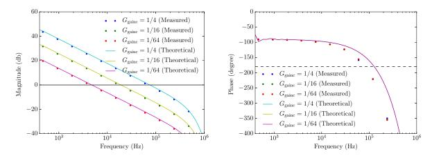
Fig. 4.24 The measured and theoretical frequency responses in the single channel loopback mode for various gain parameters
