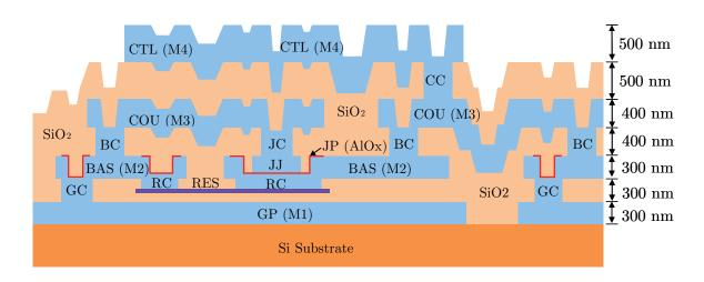
Fig. A.1 The device structure of SRL Nb Standard Process (STD3) [23]
