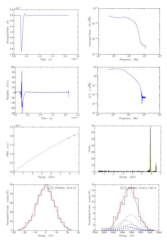
Fig. 5.14 The pulse collection result in channel 1 at 180 mK: the averaged pulse (top left), the averaged noise (top right), the template (2nd top left), the signal-to-noise ratio (2nd top right), the energy calibration curve (2nd bottom left), the energy spectrum (2nd bottom right), the baseline energy resolution (bottom left), and the energy resolution at  $MnK\alpha$  (5.9 keV).
