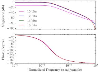
Fig. 4.12 Frequency responses of biquad low-pass filter for various fraction bits
