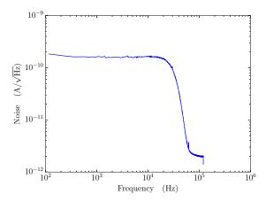
Fig. 6.4 The current noise when the TES is in the normal state at 240 mK
