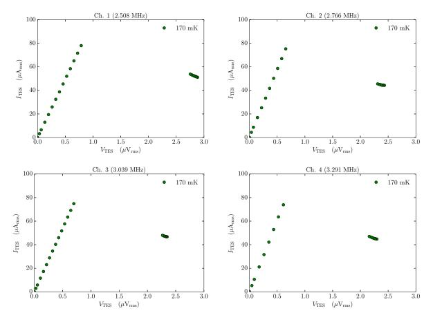
Fig. 5.15 The simultaneously measured I-V characteristics multiplexing all channels
