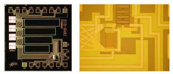
Fig. 3.11 Photomicrographs of the 4-input ISAS-G15 with inductors and capacitors: an overall view of the chip (left) and a zoomed current-summing point (right)
