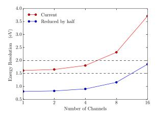
Fig. 6.3 The contribution of the readout system to the energy resolution when the system noise is reduced by half
