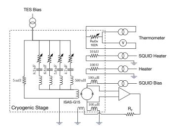
Fig. 5.3 The equivalent circuit for the cryostage setup
