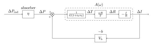
Fig. 2.7 Electrothermal feedback
