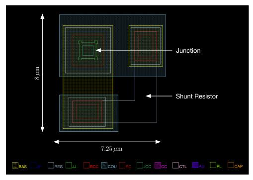
Fig. 3.1 The design of the junction and shunt resistor part
