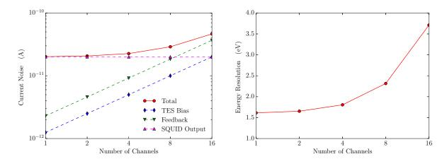
Fig. 6.2 The current noise due to the readout system (left) and the contribution to the energy resolution (right) for various number of multiplexing channels
