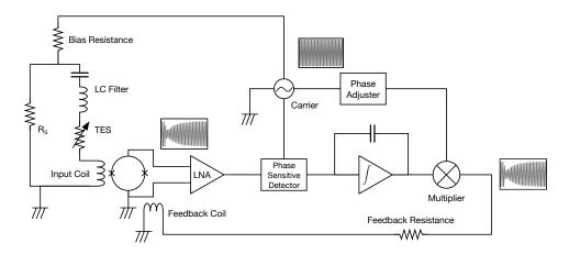
Fig. 4.6 The schematic diagram of the baseband feedback architecture. Only the single channel configuration is shown.
