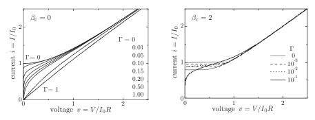
Fig. 2.12 Calculated I-V characteristic for various values of  $\Gamma$  for negligible capacitance (left) and finite capacitance (right). Adapted from Clarke and Braginski [6].
