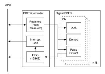
Fig. 4.17 The BBFB controller attached to the APB
