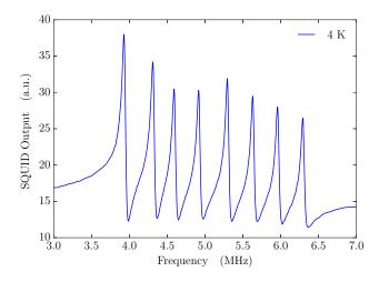
Fig. 3.19 The measured LC bandpass filter characteristic at 4 K
