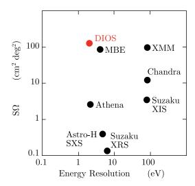
Fig. 2.3 The comparison of  $S\Omega$  for DIOS and other space missions
