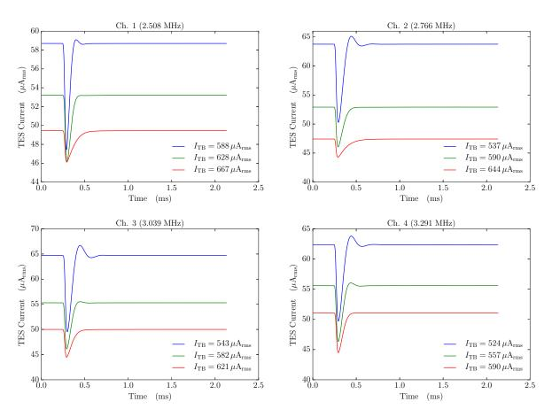
Fig. 5.12 The averaged pulses in each channel at  $150\,\mathrm{mK}$  for various TES bias currents
