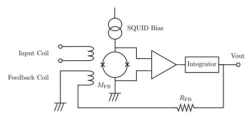
Fig. 2.19 The schematic diagram of Flux-Locked Loop (FLL)
