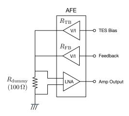
Fig. 4.30 The analog front-end measurement setup
