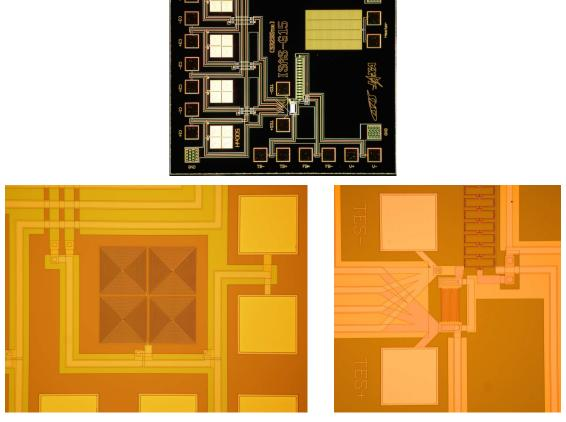
Fig. 3.10 Photomicrographs of the 4-input ISAS-G15 with inductors: an overall view of the chip (top), a zoomed inductor (bottom left), and a zoomed current-summing point (bottom right)
