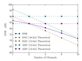
Fig. 4.23 The obtained signal-to-noise ratio in the loopback test
