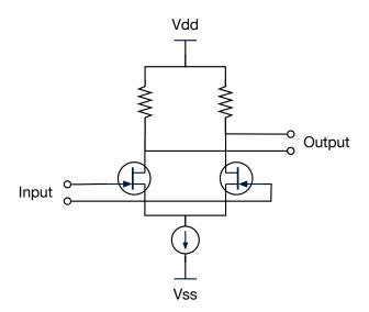
Fig. 4.28 The circuit schematic of typical FET differential amplifier
