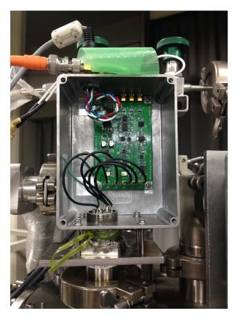
Fig. 5.6  $\,$  The analog front-end directly mounted to the refrigerator port
