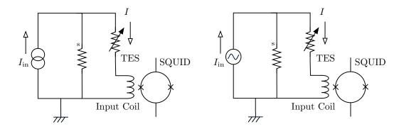
Fig. 4.1 TES biasing with DC-current (left) and AC-current (right)
