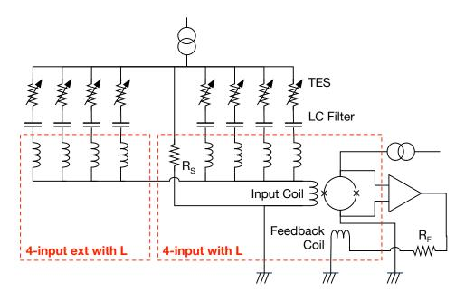
Fig. 3.6 Equivalent circuits for the 4-input SQUID chip with inductors and the 4-input extension chip with inductors
