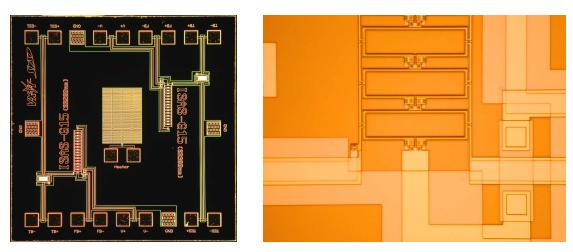
Fig. 3.9 Photomicrographs of the fabricated ISAS-G15: an overall view of the chip (left) and a zoomed SQUID (right)
