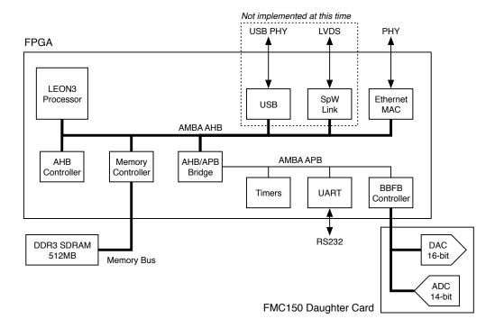
Fig. 4.16 SoC design with LEON3 microprocessor
