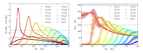
Fig. 3.17  $\partial V/\partial \Phi_{\rm in}$  and the dynamic resistance in 0–0.5  $\Phi_0$  of ISAS-G15 for various values of bias current. The dashed lines show the design goals, while the solid lines show the design requirements.
