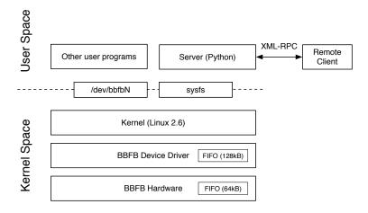
Fig. 4.18 Application stack on the SoC
