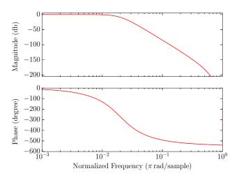
Fig. 4.13 Frequency response of 3rd-order low-pass filter
