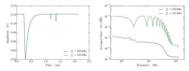
Fig. 4.25 The averaged pulses (left) and the averaged noises (right) for various spacing frequencies
