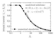
Fig. 2.11 Calculated hysteretic I-V characteristics for various values of  $\beta_{\rm C}$  (left) and the return critical current vs.  $\beta_{\rm C}$  (right). Adapted from Clarke and Braginski [6].
