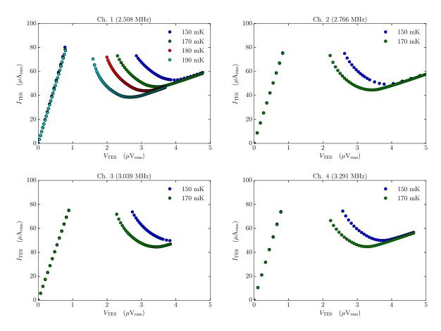
Fig. 5.11 The measured I-V characteristics of each channel in non-multiplexing
