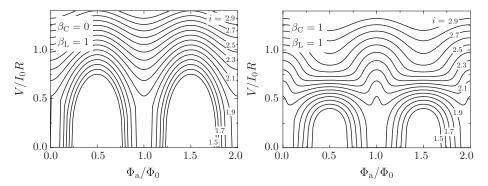
Fig. 2.16  $\Phi$ -V characteristic:  $\beta_{\rm C} = 0$  (left) and  $\beta_{\rm C} = 1$  (right). Adapted from [6].
