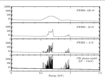
Fig. 2.2 The simulated X-ray spectra of an optically-thin thermal plasma with  $kT=3\,\mathrm{keV}$  for various energy resolutions
