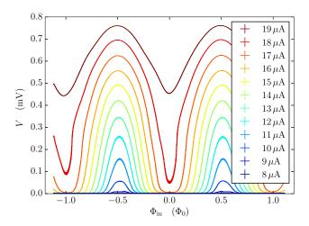
Fig. 3.16 The  $\Phi$ -V characteristics of ISAS-G15 for various values of bias current
