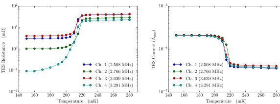
The measured R-T characteristics (left) and the TES current during the R-T measurement (right)
