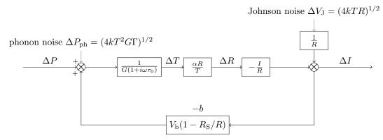
Fig. 2.8 Electrothermal feedback with intrinsic noises
