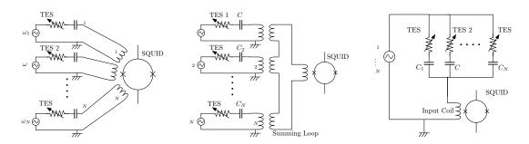
Fig. 2.22 Signal summing methods in FDM: flux summing (left), voltage summing (middle), and current summing (right)
