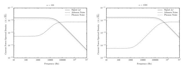
Fig. 2.9 Examples of noise current power spectral density. The left plot shows when  $\alpha = 100$ , while the right shows when  $\alpha = 1000$ .
