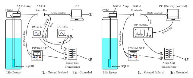
Fig. 3.13 Experimental setups for  $\Phi$ -V measurements (left) and noise measurements (right)
