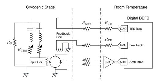
Fig. 4.27 A typical experimental setup for a TES multiplexed readout
