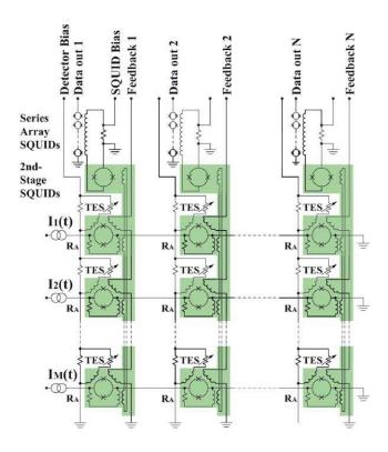
Fig. 2.21 The schematic diagram of the SQUID TDM architecture. Adapted from Irwin et al. [18].
