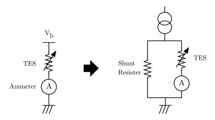
Fig. 2.6 Constant voltage biasing (left), and constant voltage biasing using a shunt resistor (right)
