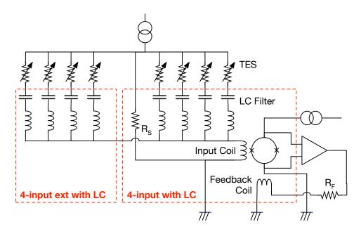
Fig. 3.8 Equivalent circuits for the 4-input SQUID chip with built-in LC filters and the 4-input extension chip
