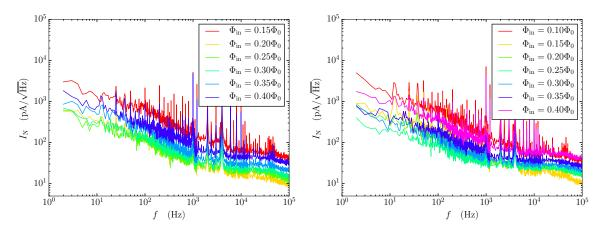
Fig. 3.18 Equivalent input current noises of ISAS-G15 in the open loop for various  $\Phi$  offsets:  $I_{\rm b}=16\,\mu{\rm A}$  (left) and  $I_{\rm b}=17\,\mu{\rm A}$  (right)
