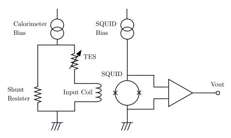
Fig. 2.18 TES readout using SQUID
