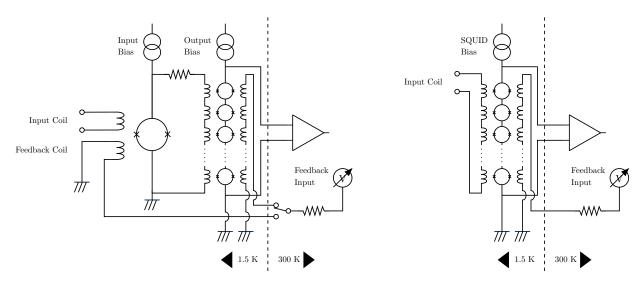
Fig. 2.20 The TES readout using the SQUID array: the two-staged SQUID (left), and the SQUID series array (right)
