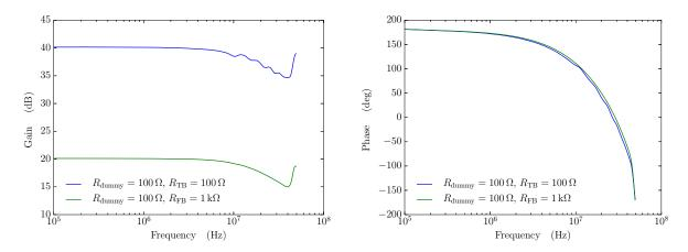
Fig. 4.31 The measured gain (left) and phase (right) of the analog front-end
