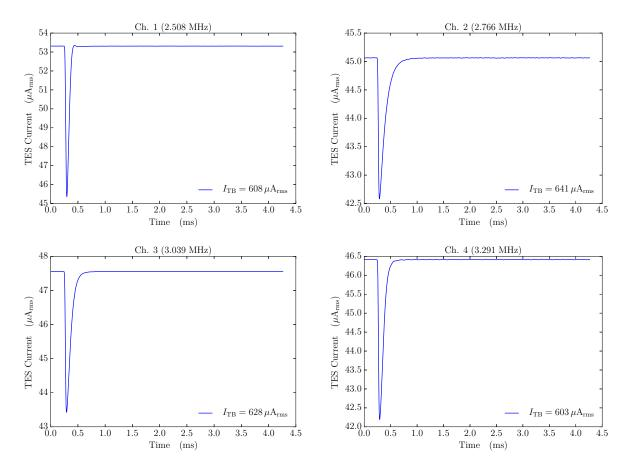
Fig. 5.16  $\,$  The averaged pulses in each channel at  $170\,\mathrm{mK}$  for various TES bias currents
