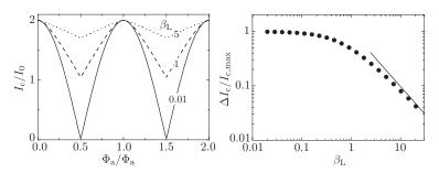
Fig. 2.15 Critical current of the dc SQUID vs. applied magnetic flux for various values of  $\beta_{\rm L}$  (left) and the modulation depth vs.  $\beta_{\rm L}$  (solid line is  $\beta_{\rm L}^{-1}$ ) (right). Adapted from Clarke and Braginski [6].
