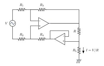
Fig. 4.29 The circuit schematic of the V/I converter based on the op-amp differential amplifier
