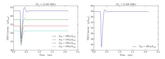
Fig. 5.13 The averaged pulses in channel 1 at  $180\,\mathrm{mK}$  (left) and  $190\,\mathrm{mK}$  (right) for various TES bias currents
