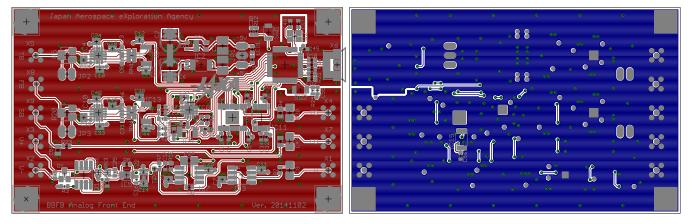
Fig. C.2 Full-scale PCB layouts of BBFB analog front-end: the component side (left) and the solder side (right)
