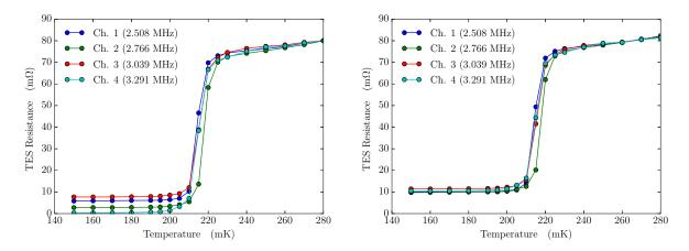
Fig. 5.10 The TES shunt resistor adjusted R-T (left) and the TES bias level adjusted R-T (right)
