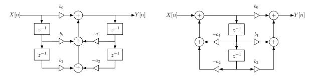
Fig. 4.11 Biquad filter implementations: direct form 1 (left) and direct form 2 (right)
