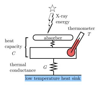
Fig. 2.4 A schematic view of an X-ray microcalorimeter
