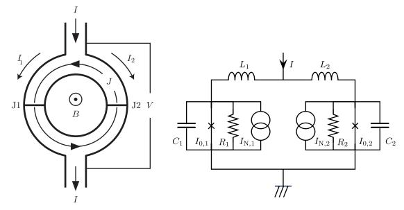
Fig. 2.13 The dc SQUID: the schematic diagram of dc SQUID (left) and the equivalent circuit of dc SQUID
