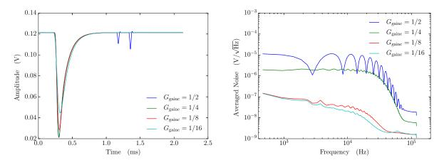
Fig. 4.26 The averaged pulses (left) and the averaged noises (right) for various gain parameters ( $f_s = 125\,\mathrm{kHz},\,G_\mathrm{div} = 1/4$ )
