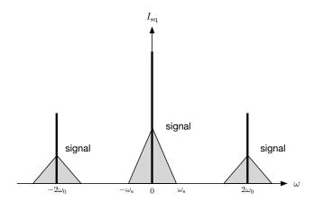
Fig. 4.4 The demodulated signal power spectrum using the phase detection method
