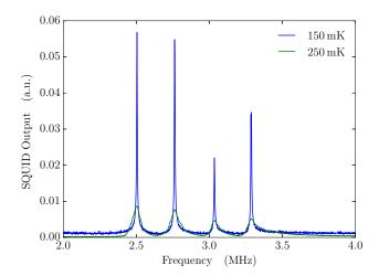
Fig. 5.8 The LC filter characteristics at 150 mK (TES super) and 250 mK (TES normal)
