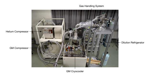
Fig. 5.1 The dry <sup>3</sup>He-<sup>4</sup>He dilution refridgerator
