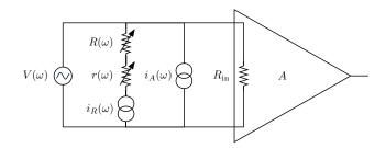
Fig. 4.5 Equivalent noise circuit for AC-biased microcalorimeter
