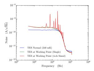
Fig. 6.5 The current noises for various TES states
