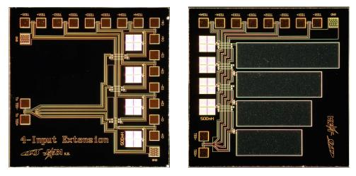
Fig. 3.12 Photomicrographs of the 4-input extension chips: an extension with inductors (left) and an extension with inductors and capacitors (right)
