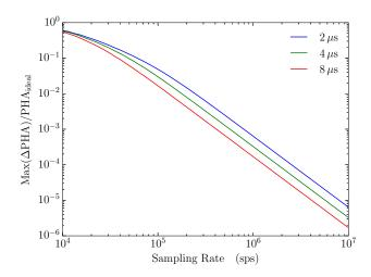
Fig. 4.14 Dispersion of pulse heights (PHA) vs. sampling rates for various pulse rise times
