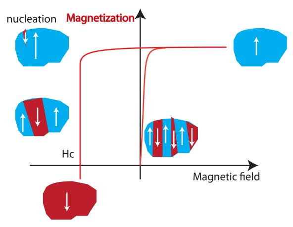
FIGURE 1.4: Schematic picture of demagnetization curve based on the nucleation process.
