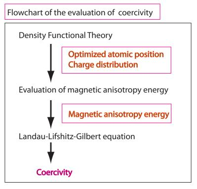
FIGURE 2.1: Flowchart of evaluation of coercivity
