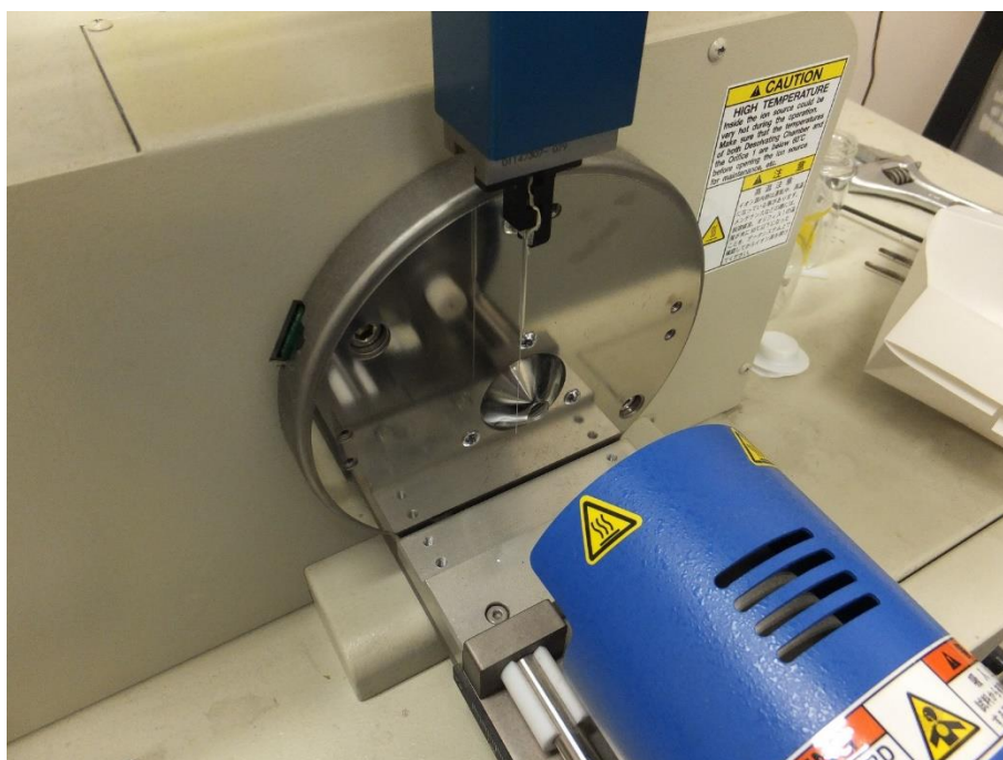
Figure 2-4. Ionization by DART-MS with auto-sampler
