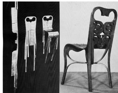
Thonet experimental chair from laminated veneers, process shown on right, 1880 (CW)
