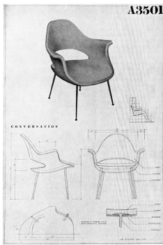
Organic Design Competition drawing of the armchair submitted by Saarinen and Eames, with plywood shell, rubber-weld joint, and aluminum legs (EN)
