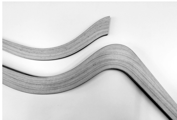
Fig. 3.3.5-3 Example of the irregular thickness moulded plywood by Tendo Mokko today, used in some designs of chair legs
