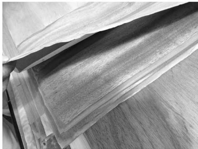
small strips of veneers (0.25 - 1.0mm), with industrial washi paper backing applied
