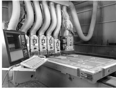
CNC router prepares MDF forms
