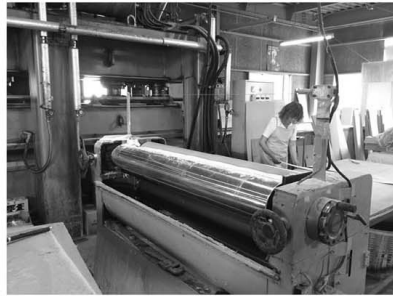
roller machine applies glue onto veneers
