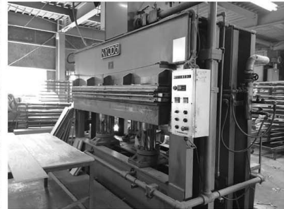
hydraulic heated veneer press
