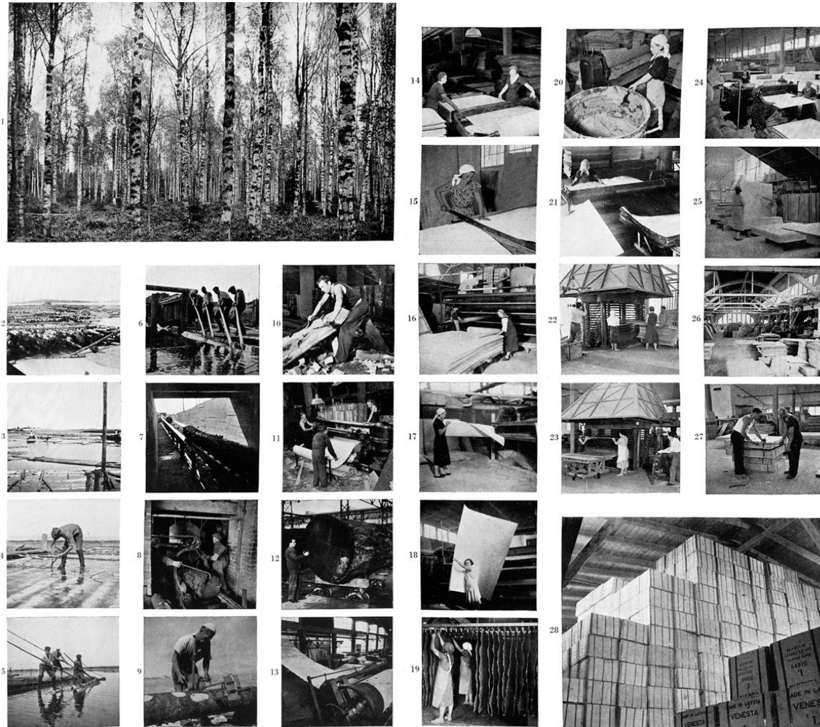
Fig. 2.3.10 Stills from an instructional film, “Plywood in the Making” published in the Architectural Review from 1936 shows the process of birch plywood production typical in northern Europe: 90 1. Selection of trees; 2. Logs are sorted by size, quality, and ownership; 3. Logs transported to the manufacturer; 4-6. Logs being punted into the sawmill; 7-9. Sorted and cut into appropriate lengths; 10. Bark is roughly sliced off; 11. The wet log is peeled on the veneer lathe; 12-13. Gaboon (West African hardwood, also known as Okuome) logs provide a scale comparison to the birch; 14-15. Cutting by a slicer into required lengths, while smaller strips are connected with paper tape; 16. The wet sheets of veneer are placed onto the racks of drying kiln; 17-19. Veneers after kiln dried; 20. The “liquid cement” – a compound of blood albumen and casein – kept in the heated cauldron at the right consistency; 21. Veneers fed through cementing rollers; 22. Stacked veneers are subjected to regulated pressure and increasing heat; 23. Flat and rigid sheets of plywood
