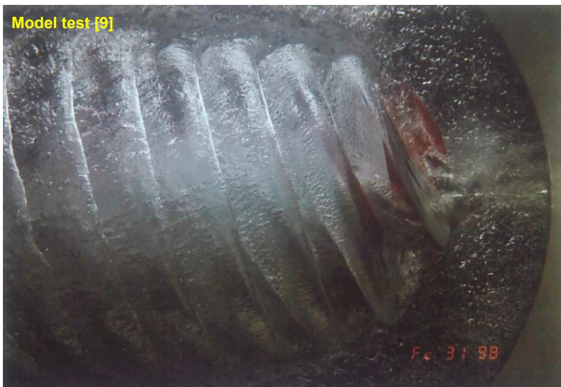
Fig. 3.22 Comparison of thickness and pitch of ventilation between CFD and model test. ( J=0.8 )
