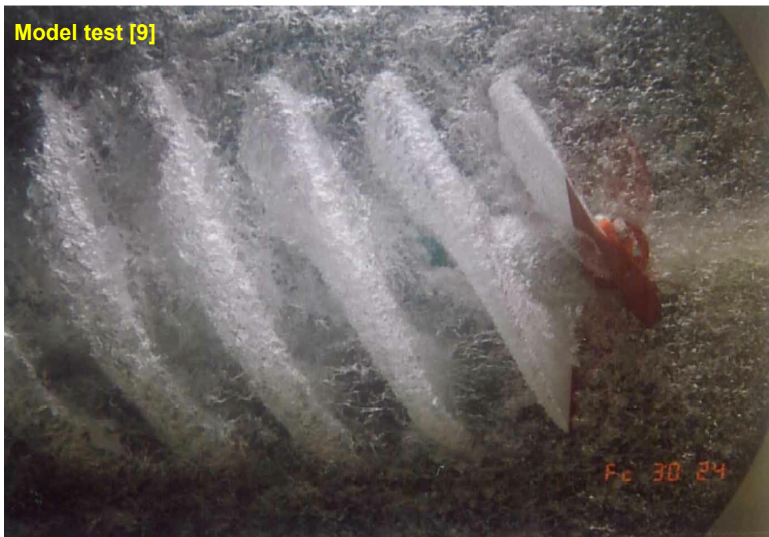
Fig. 3.24 Comparison of thickness and pitch of ventilation between CFD and model test. ( J=1.0 )
