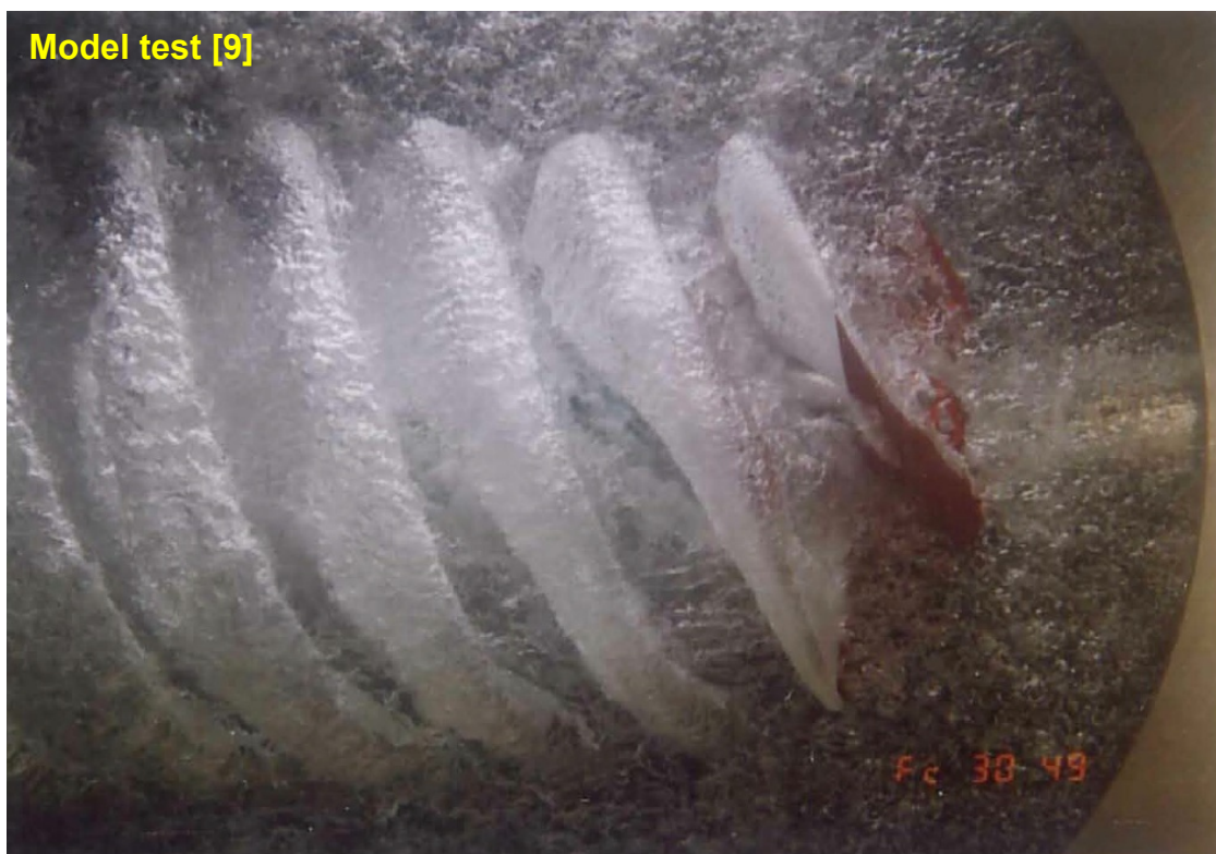
Fig. 3.23 Comparison of thickness and pitch of ventilation between CFD and model test. ( J=1.0 )
