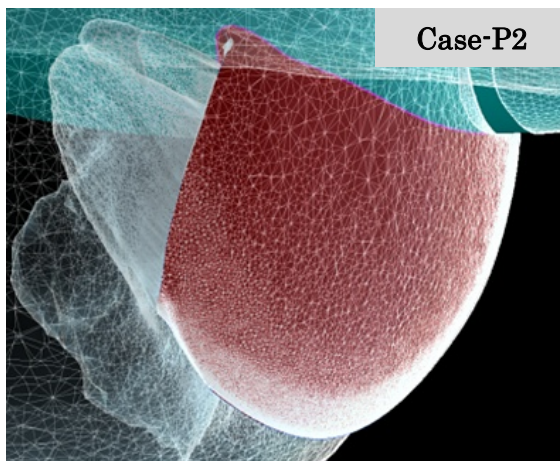
Fig. 2.22 Comparison of ventilation patterns at J=0.40 .
