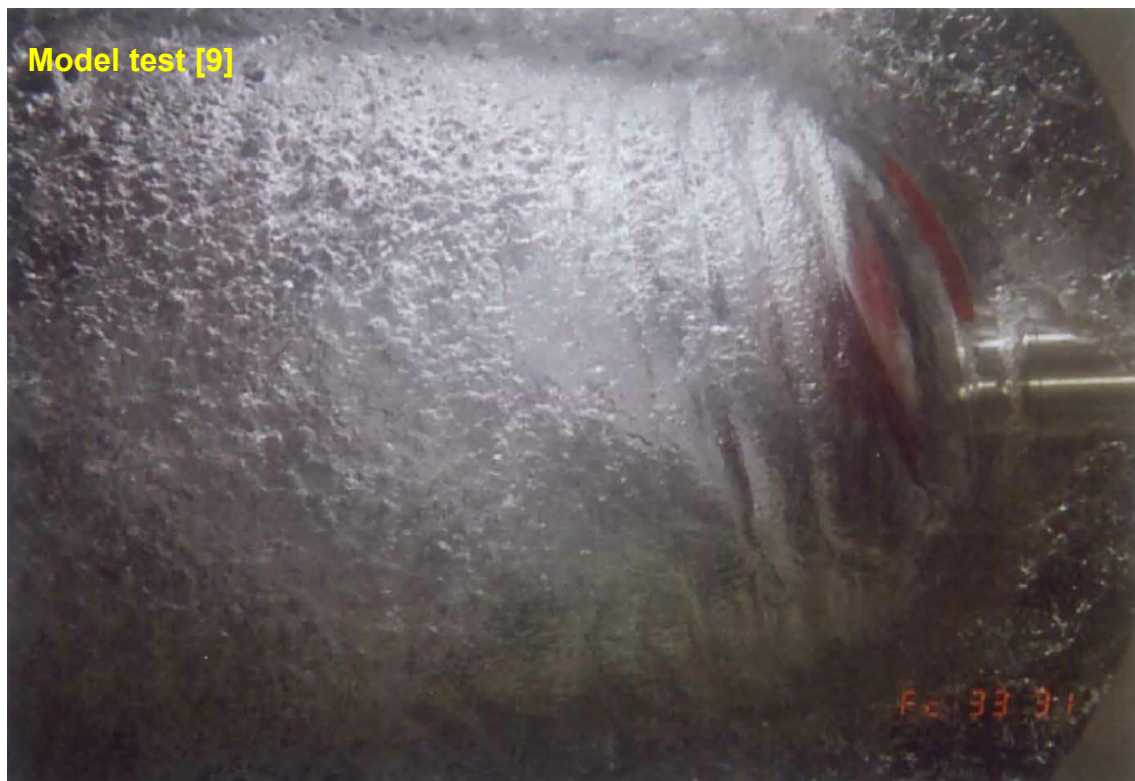
Fig. 3.20 Comparison of thickness and pitch of ventilation between CFD and model test. ( J=0.4 )
