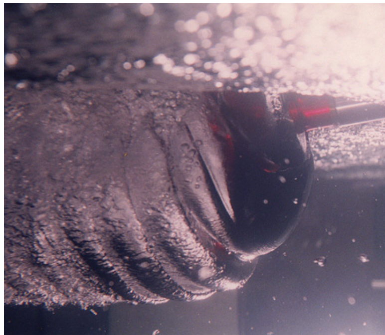
Fig. 1.2 Observation of ventilation pattern in the model test.
