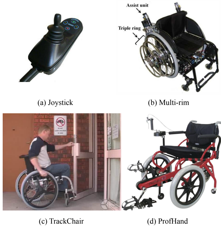
Figure 5.1: Previous one-handed wheelchairs ( Sakai and Yasuda, 2013 )( Profhand, 2013 )
