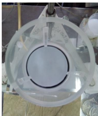
Fig. 6.3 Assembly of instruments related to making the MFC/PAM composite sheets through the filtering process.
