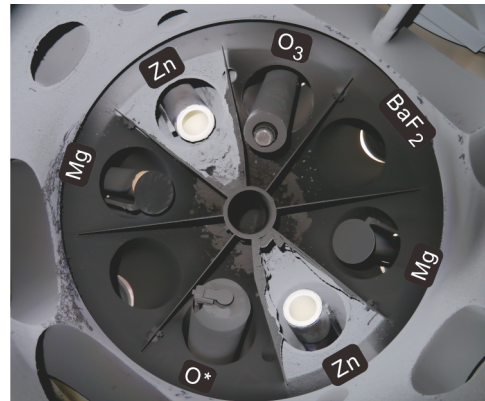
Figure 3.3: Photograph of inside the MBE apparatus showing the base partitioned into 8 sections, corresponding to the 8 ICF152 ports which host the source materials and view ports. Individual components are labelled.
