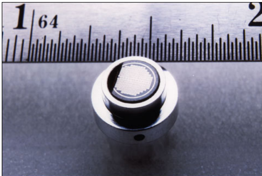
Fig. 3-17 Official photograph of HFM heat flux sensor [84]
