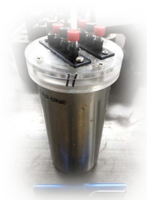
Fig. 3-22 Cold junction apparatus equipped with wiring terminals (photographed by K. Yamaguchi)
