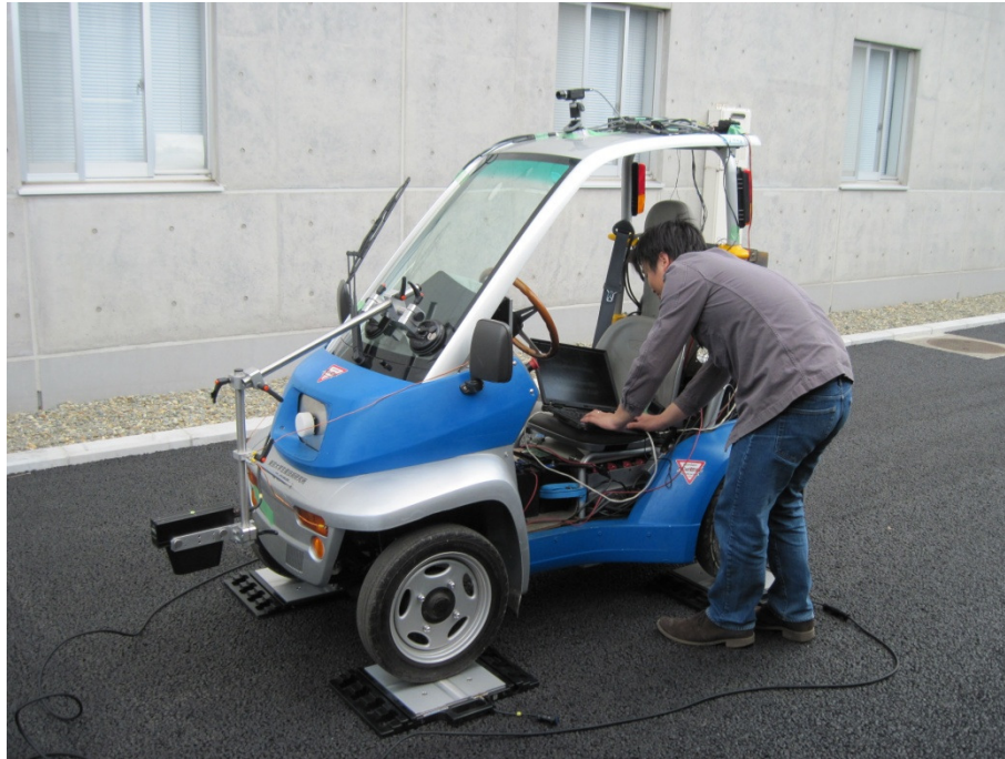
Photo 3: Preparing the experiment beside the garage (Spring 2012). The vehicle is placed on four load sensors which are used to measure the weight (at each wheel) of the vehicle. By this way, we can find the center of gravity of the vehicle.
