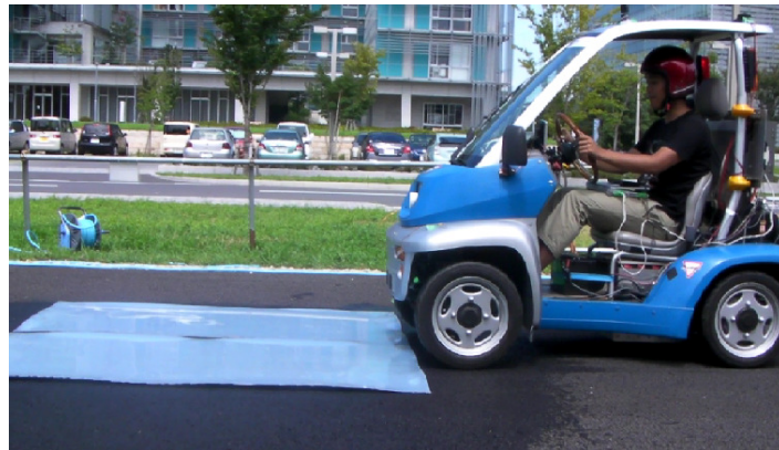
Fig. 5.24 Traction control on slippery road.
