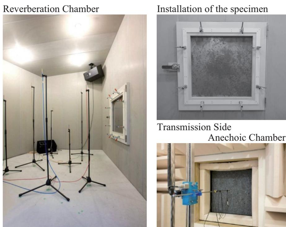
Fig. 5.50: Measurement chamber and the condition of material installation.
