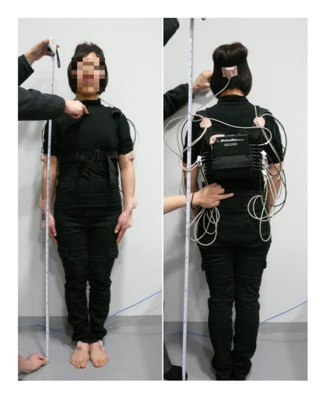
Figure A.2: Magnetic motion capture system from Ascension. To capture the Don-pan dance, totally 15 markers are attached to the dancer in chapter 3.
