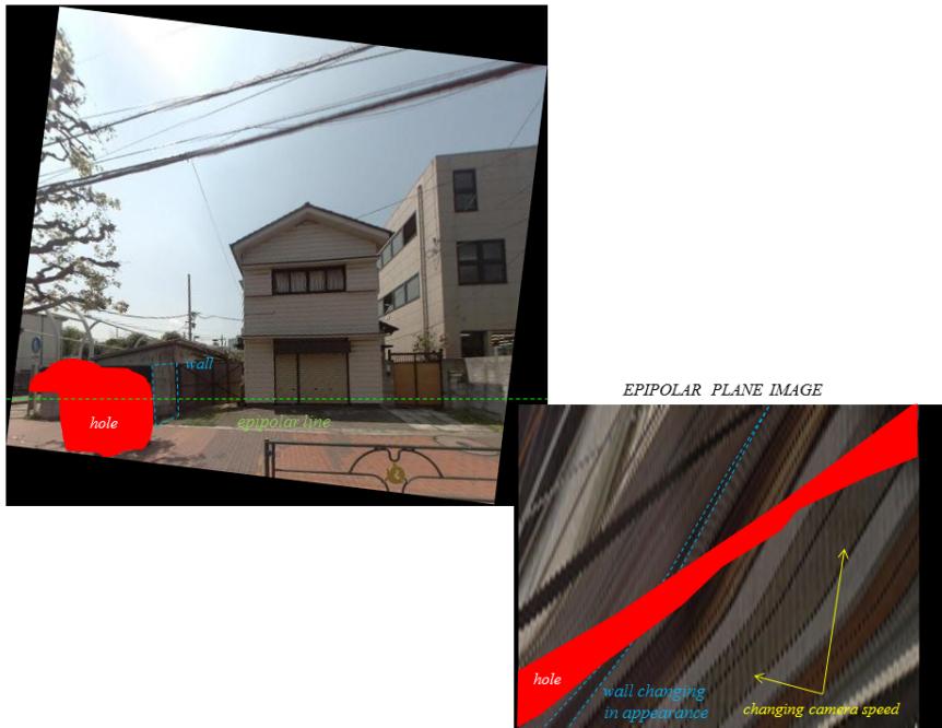
Figure 5.2: Sequence with a wall changing its appearance on either side of the hole with the camera changing its speed at the same time.
