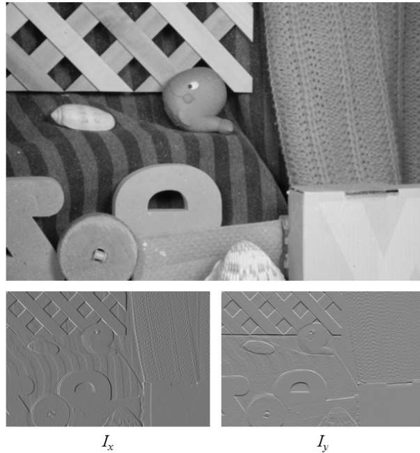
Figure 4.5: Image gradients I_x and I_y of the top image in the x and y directions, respectively.
