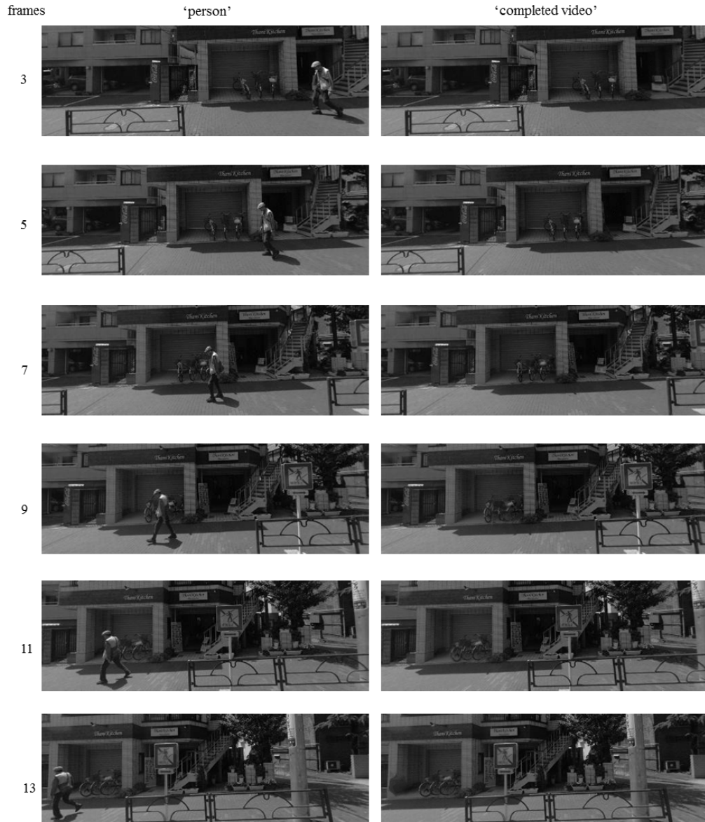
Figure 5.27: Representative frames of the result of completion of a real street video where the pedestrians are removed.
