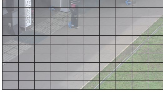
Figure 2.5: An example of dividing a scene into 10 \times 10 unit regions ( K = 100 ). These regions serve as the smallest unit to construct each region.
