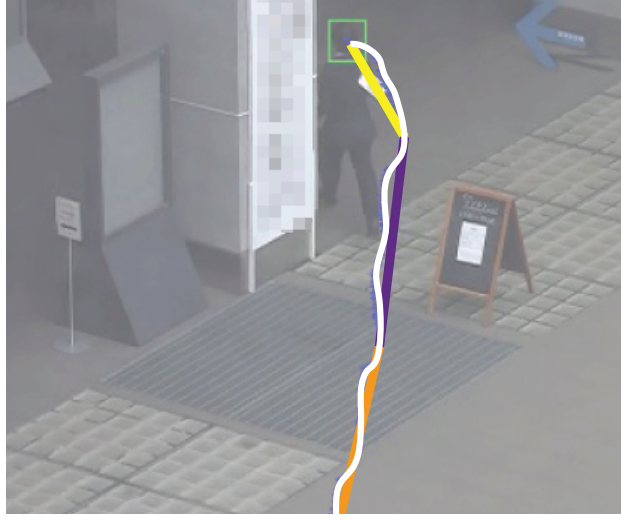
Figure 2.4: An example of polyline simplification. The curved line shows a tracking result and straight lines show the result of polyline simplification.
