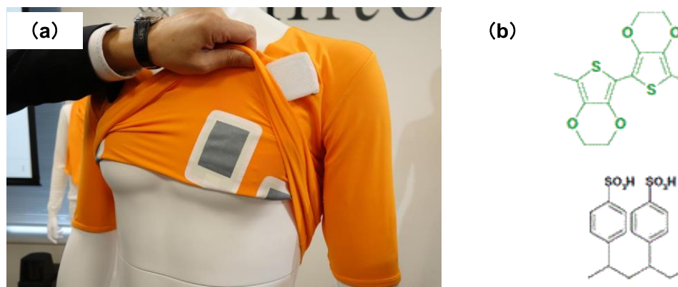
Figure 2.2 ECG sensing T-shirt w/ Poly(3,4-ethylenedioxythiophene)-poly(styrenesulfonate) (PEDOT/PSS). (a) Electrode on T-shirt (gray part) [35]. (b) Chemical structure of PEDOT/PSS [36].
