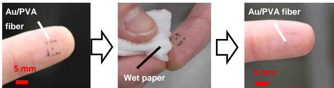
Figure 6.13 Sequence of Au/PVA fiber removal test
