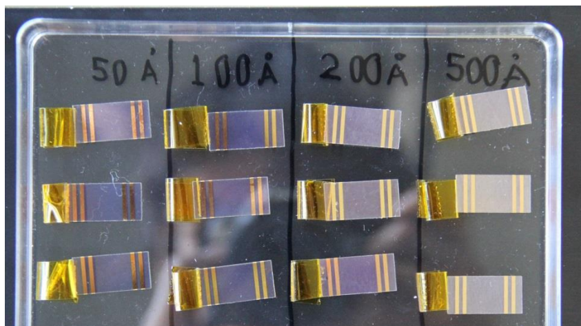
Figure 5.16 Au covered PVA mesh electrode, Au thickness is 5, 10, 20 or 50 nm
