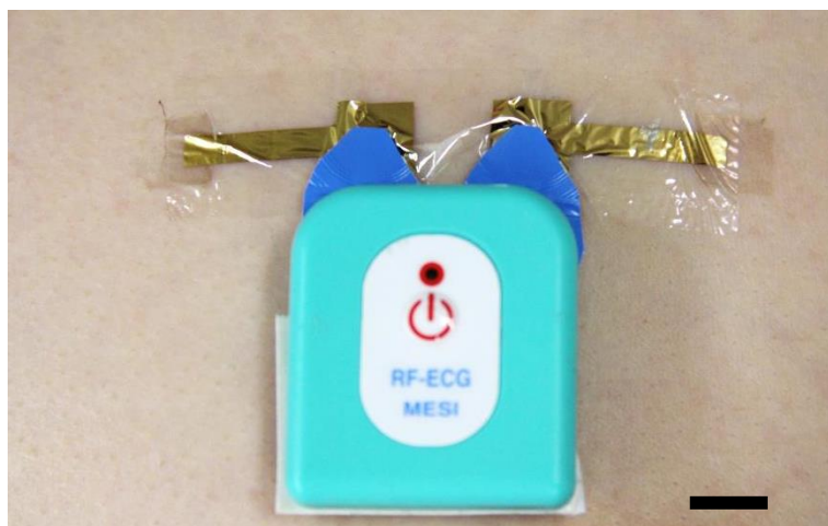
Figure 6.16 Au covered PVA mesh electrode and wireless ECG sensor set on a human body.
