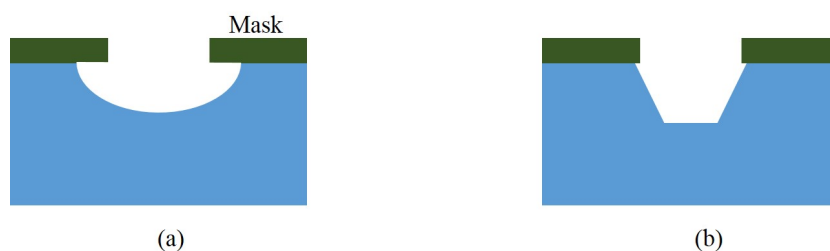
Fig.4.1 (a)The isotropy etching. (b)The anisotropy etching.
