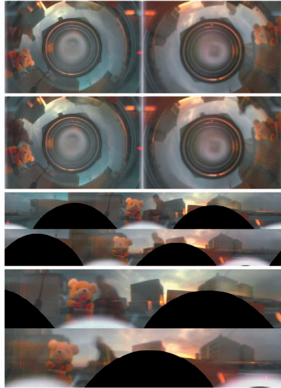
Fig. 27. Image capture with linear polarization separation in the low-speed shutter mode. Shown in the first and second rows are the original images for frame n and frame n + 1 , respectively (left-eye images on the left column and right-eye images on the right column). Shown in the next two rows are the converted images (left-eye images on the upper side and right-eye images on the lower side).
