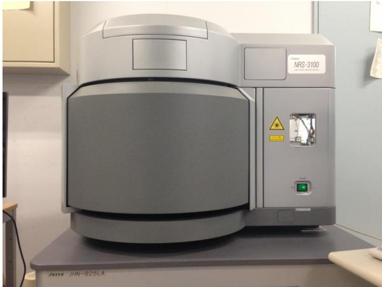
Figure 2.5 Picture of apparatus for Raman spectroscopy NRS-3000.
