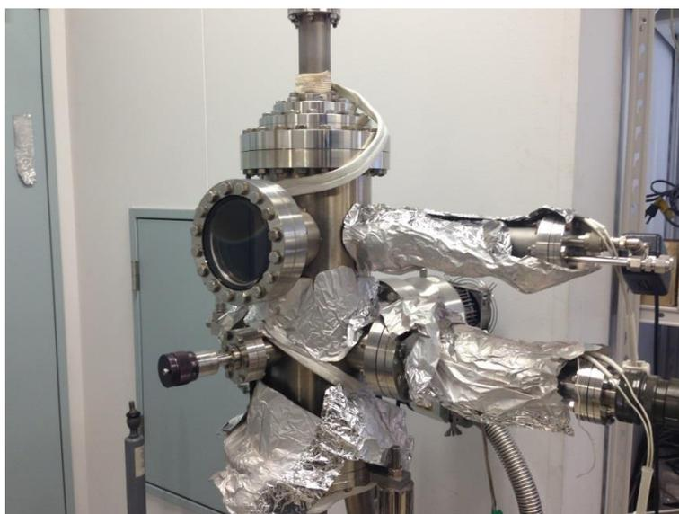
Figure 2.1 Picture of the metal deposition chamber
