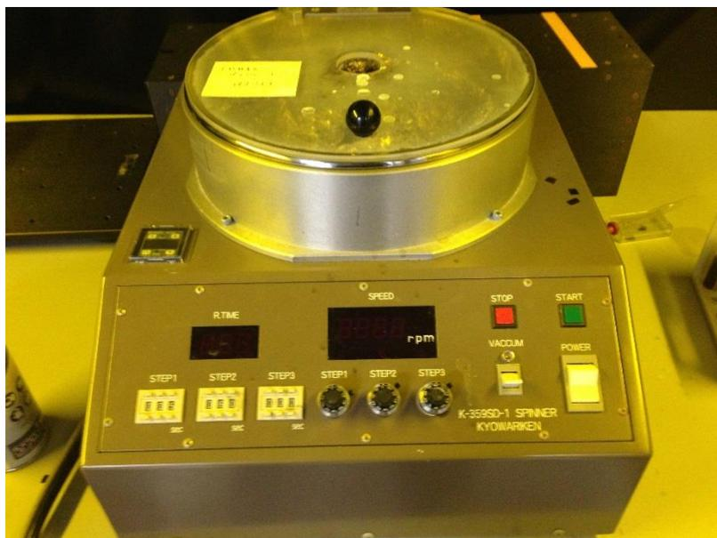
Figure 2.11 Picture of spin coater K-359SD-1.
