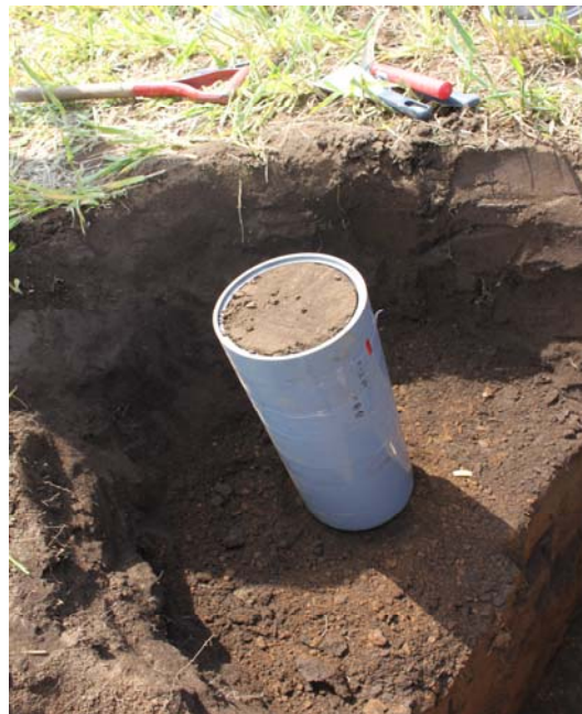
Fig. 5 Undisturbed soil columns sampling
