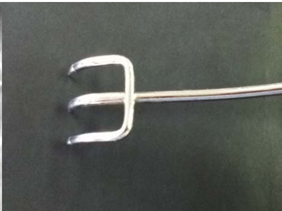
Fig. 6 Leaf compost (after crushed) applied to the soil (a); Garden helper used to simulate tillage operation in the laboratory (b)
