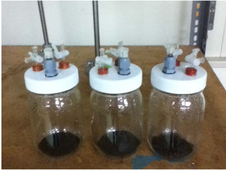
Fig. 10 Incubation bottles used for the measurement of the respiration rate associated with aggregates
