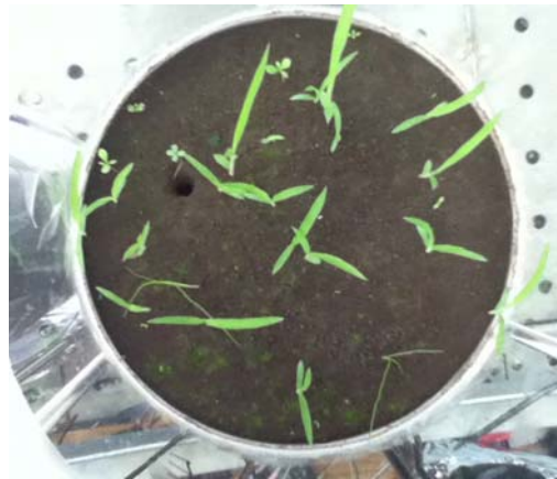
Fig. 12 Soil column under no-tillage-with macropore (RNT-M) treatment. A macropore (diameter of 3 mm) was left in the soil column
