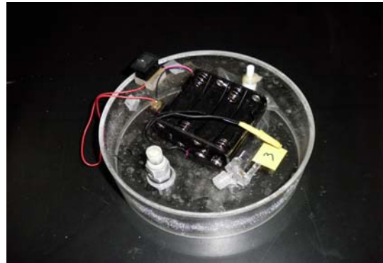
Fig. 9b The gas sampling port, the thermocouples, the porous cup and the chamber used in the incubation experiment
