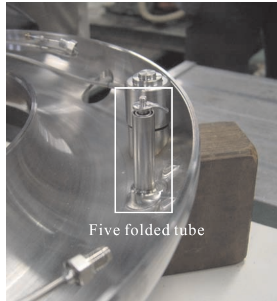
Figure A.3: Structure and Photograph of Five Folded Tube
