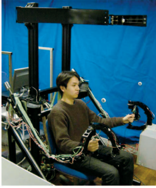
Fig. 5. The master arm of TELESAR II.
