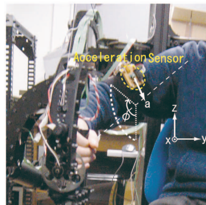
Fig. 12. Swivel angle, an acceleration sensor attached to an operator's upper arm, and its axis a .
