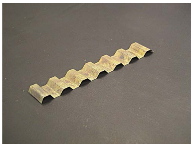
Fig. 2.12 SMA foil after shape memory treatment.
