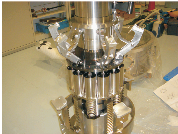
Figure 2.6: Photographic view of F-coil catcher. The catcher is opened in this photograph.
