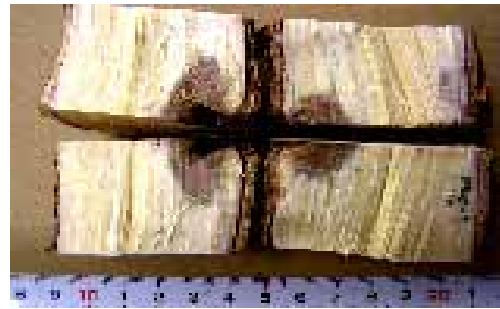
Fig.6 Wood discoloration column shape. Konara, six months after winter wounding
