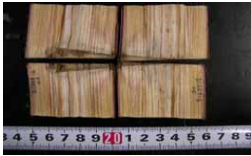
Fig.5 Wood discoloration column shape. Metasekoia, six months after autumn wounding.
