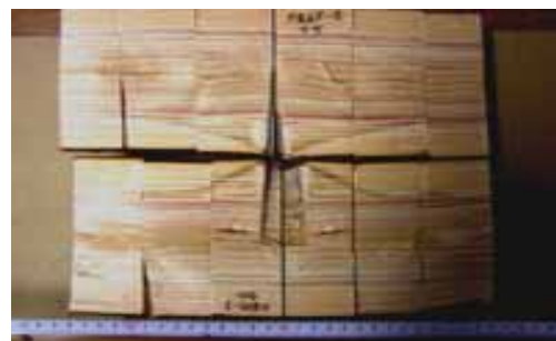
Fig.4 Wood discoloration column shape. Hinoki six months after summer wounding.
