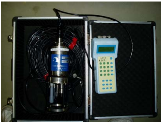
Fig. 3-6 Mobile instrument for measuring water quality
