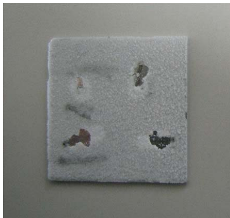
Fig.3-18 Photograph of the Jaxa Coating after the pencil hardness test (Pencil hardness H)
