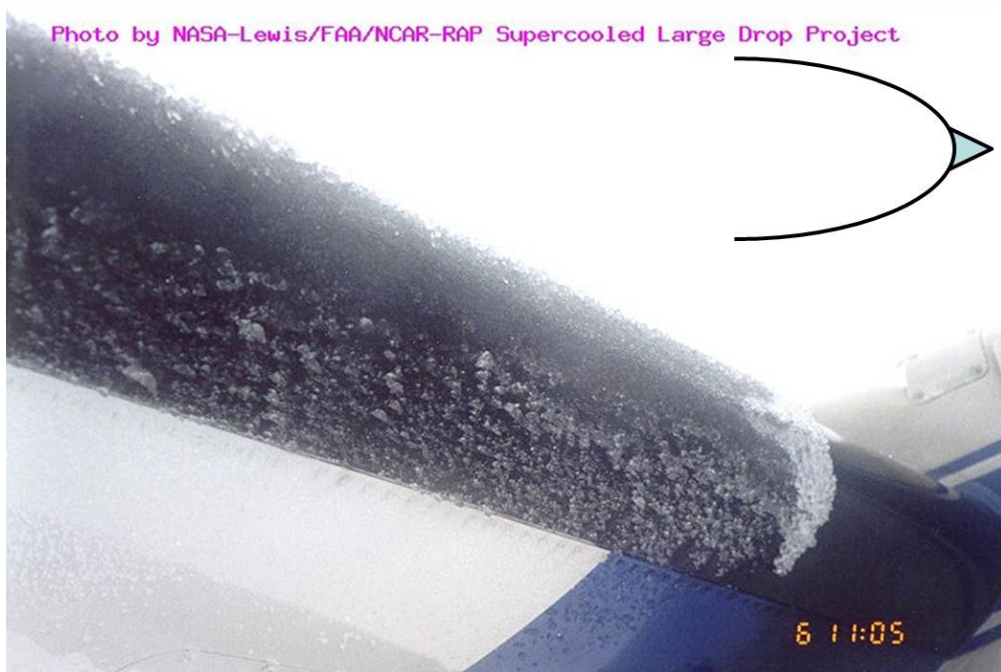
Fig.2-17 Photograph and schematic of rime ice on a leading edge of a wing (39)
